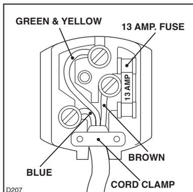
Connect the Green and Yellow (earth) wire to the terminal in the plug which is marked with the letter «E» or the earth symbol
