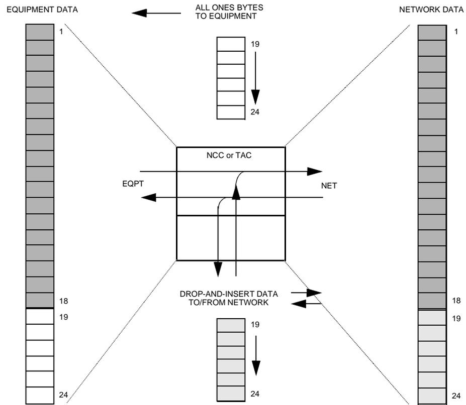
Channels 19 to 24 are available for high-speed data transmission over the network. These six channels are user-assigned to a data port of a DIU 2130 connected to the CSU. The CSU inserts the high-speed data onto channels 19 through 24 of the signal from the equipment, and then sends the composite signal to the network.
