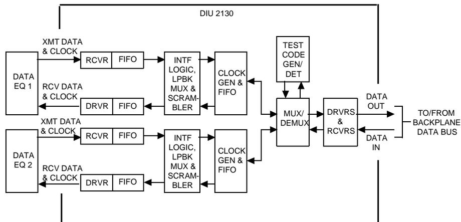
**Data Receiver** The data receiver converts the V.35, RS-449, or EIA 530 data and control signals to a format suitable for internal DIU processing.
