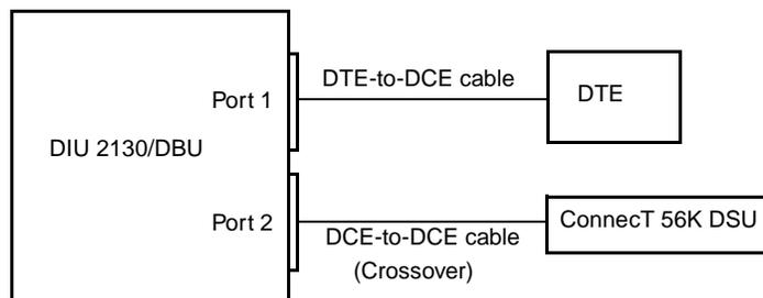
If the T1 Dial Backup Option is configured for V.35, refer to the cable part numbers in Table 5-1.
