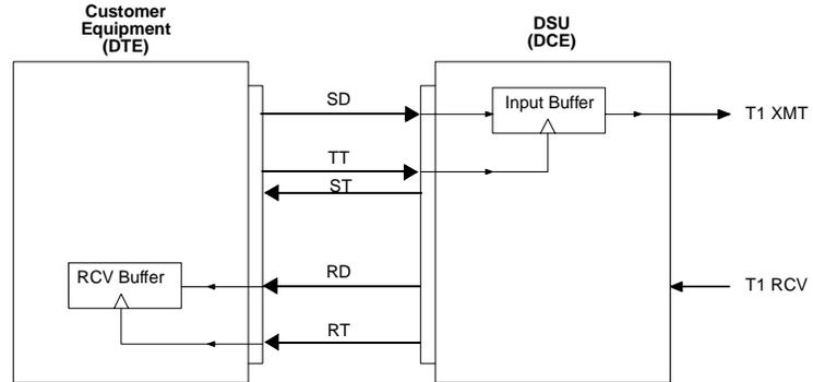
The RT signal is derived by recovering the clock from the data stream coming from the network. Since the T1 data contains overhead bits that are removed before being sent to the DTE, the frequency of this data is different than the frequency of RD. In the receive direction, the frequency is decreased from 1.544 Mbit/s to the selected interface frequency. In the transmit direction, the frequency is increased from the selected interface frequency to 1.544 Mbit/s. (Figure 7-5)
