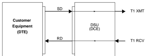
The SD and RD signals have associated clock signals called Terminal Timing (TT) and Receive Timing (RT). The DIU's input buffer may use the TT signal to clock in SD. The customer's DTE receive buffer uses the RT signal to clock in RD (Figure 7-4).
