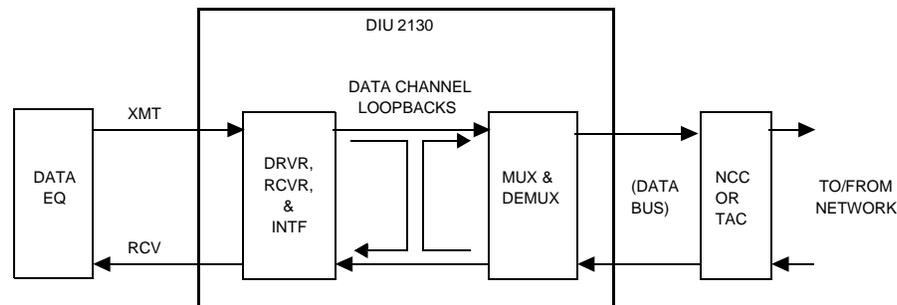
The DIU data channel loopback can be activated and deactivated on either data channel. When this loopback is activated, only the selected data channel is tested. The other data channel continues to operate normally and transmission service is not affected.
