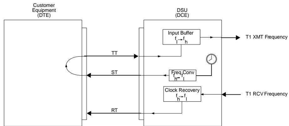
If the Far End is looped timed, then T1 XMT Frequency is = T1 RCV Frequency
