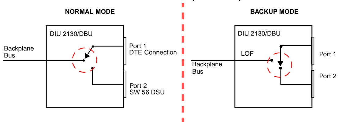
The DTR control lead of the DCE attached to Port 2 of the DIU 2130/DBU is used to initiate the call to the dial backup circuit. The handshake lead Carrier Detect (CD) is monitored in the answer mode at the central site. Backup mode initiates when:
