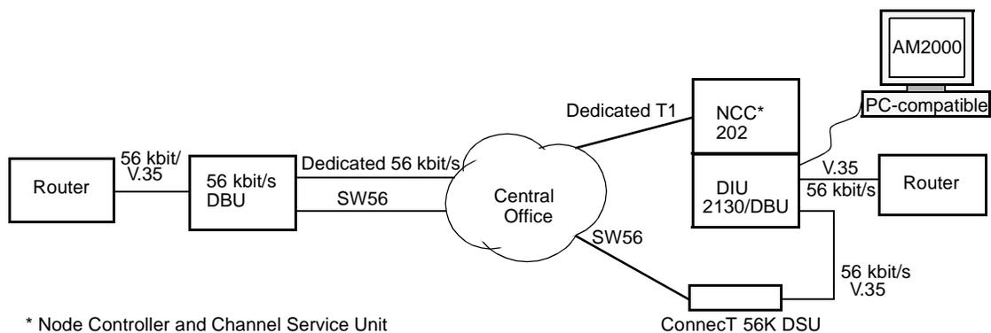
This T1 Dial Backup Option is an EPROM upgrade or download upgrade to the Verilink Data Interface Unit (DIU) 2130 plug-in module. The upgraded plug-in module is designated as the DIU 2130/DBU.
