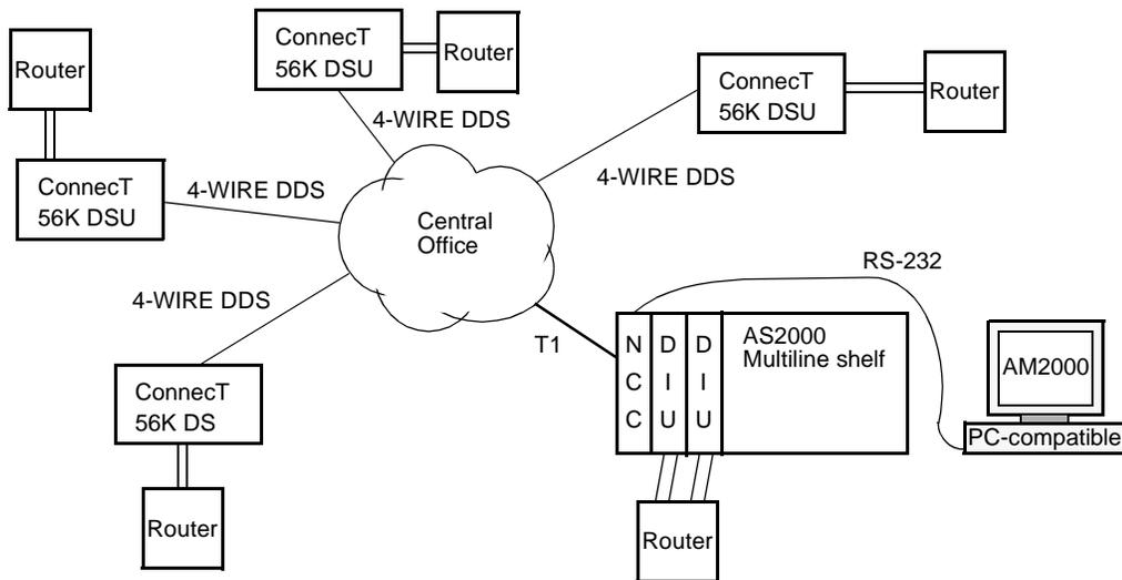
The routers are each connected to the network by ConnectT 56K DSUs. Each port of a DIU 2130/DDS supports one ConnectT 56K DSU.
