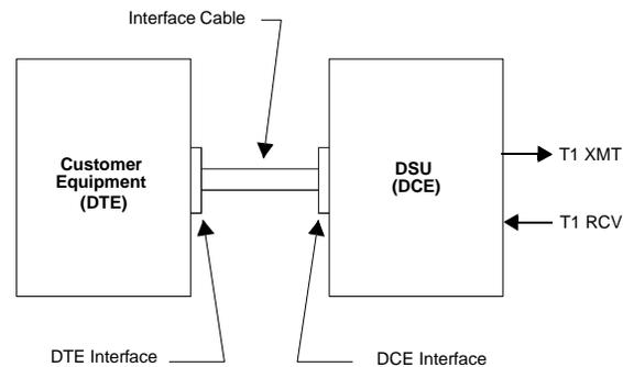
The DIU 2130 supports three types of (DTE) interfaces: ITU-T V.35, RS-449/422, and EIA 530. The RS-449/422, EIA 530, and V.35 interfaces are logically equivalent. The only difference between the three are their electrical interface characteristics (voltage levels) and connectors (Figure 7-2).
