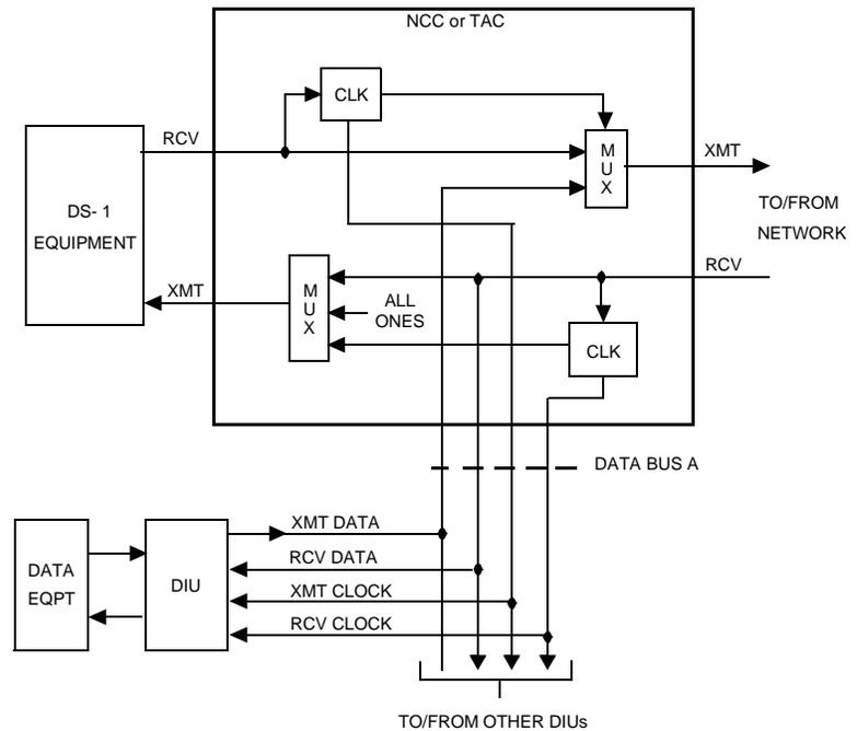
In the opposite direction of transmission, the CSU passes the incoming T1 signal to the DIUs over data bus A. The equipment-side multiplexer of the CSU also routes the incoming network signal to the DS1 equipment. In addition, it inserts all-ones idle code bytes into the DS0 channel time slots assigned to the DIUs, and sends this data to the DS1 equipment.
