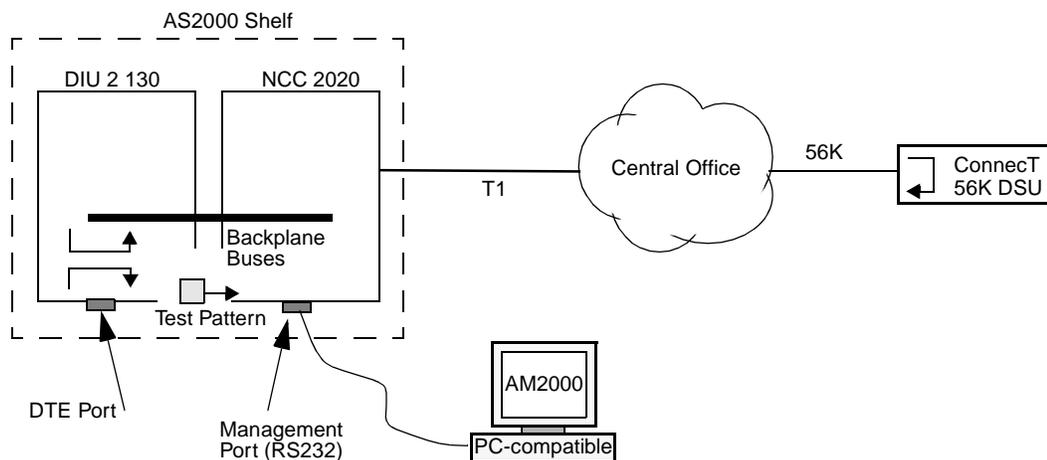
In this example, a DIU 2130 with DDS capability is connected to a ConnecT 56k DSU at the far end. To test the network circuit, a remote loop-back is first activated. In a DDS circuit to a ConnecT 56, either a DDS latching loop or a V.54 loopback option can be used to perform the remote loop-back.
