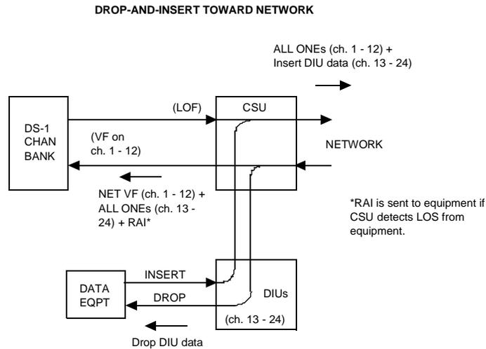
When the CSU detects an LOF from the equipment, the DIUs perform channel conditioning operations on the associated data equipment. Each DIU negates the CTS, DSR, and DCD handshaking signals to the associated customer data equipment (if not configured by the user to permanently assert these signals). It also sends all-ones idle bytes to the data equipment.
