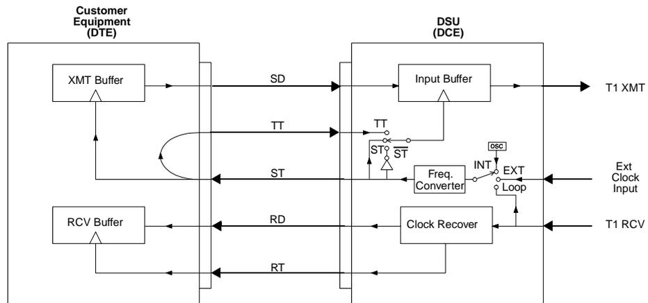
ST controls the exact bit rate at which data is transmitted toward the network on the DTE interface.
