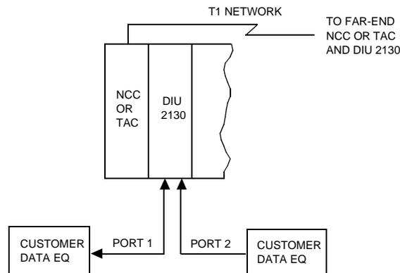
Up to twelve DIUs and one NCC 2020, SCC 2020, or TAC 2010 provide carrier network access and T1 transmission for high-speed data applications. If using the DIU 2130 DBU option at one timeslot per Port 1, then it is possible to get up to 24 DIUs per CSU module. The DIU interfaces with the associated CSU through a data bus on the shelf backplane.
