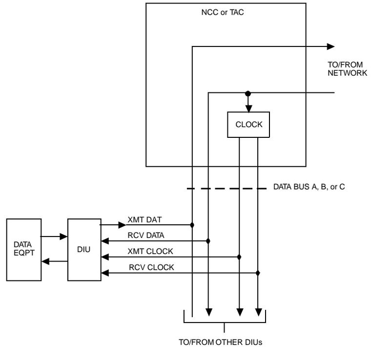
Figure 7-16 Network Timing (Drop and Insert Mode)
