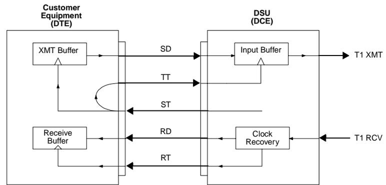
Since TT must be locked to ST, most DTE manufacturers turn ST around on TT, and TT is usually an exact duplicate of ST. (Figure 7-7)
