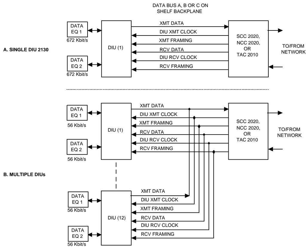
For a typical CSU/DSU configuration with multiple DIUs, up to 12 DIU 2130s can be connected to an NCC, SCC, or TAC to accommodate up to 24 data ports (Section B of Figure 1-7). In this example, each port operates at 56 kbit/s and requires one DS0 channel on the T1 network.
