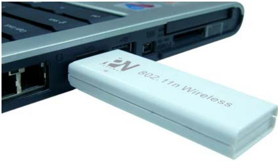
1. Please insert the wireless network card into an available USB 2.0 port of your computer. You can insert the card when the computer is power off or on.
