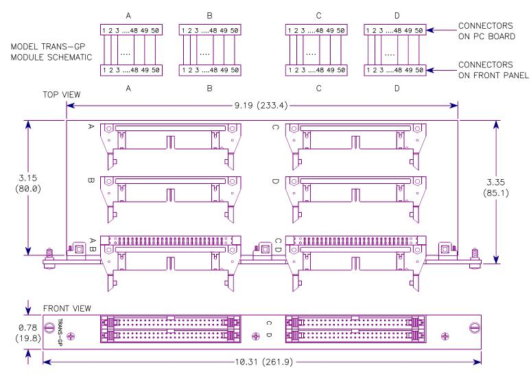
TRANS-GP MECHANICAL DIMENSIONS AND SIMPLIFIED SCHEMATIC
