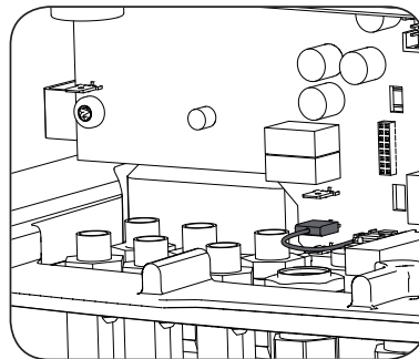
Ground connection of the positive pole (J8)
