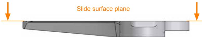
In addition, when grinding, you must make sure that the inclination of the cutting surface in the direction of the blade arm movement is not changed. Check the incline and smoothness of the ground surface, using a suitable measuring tool.
