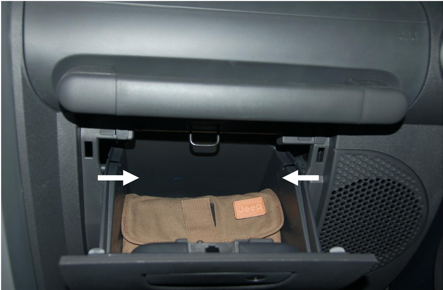
Remove glove box. Push in on both sides and set aside.
