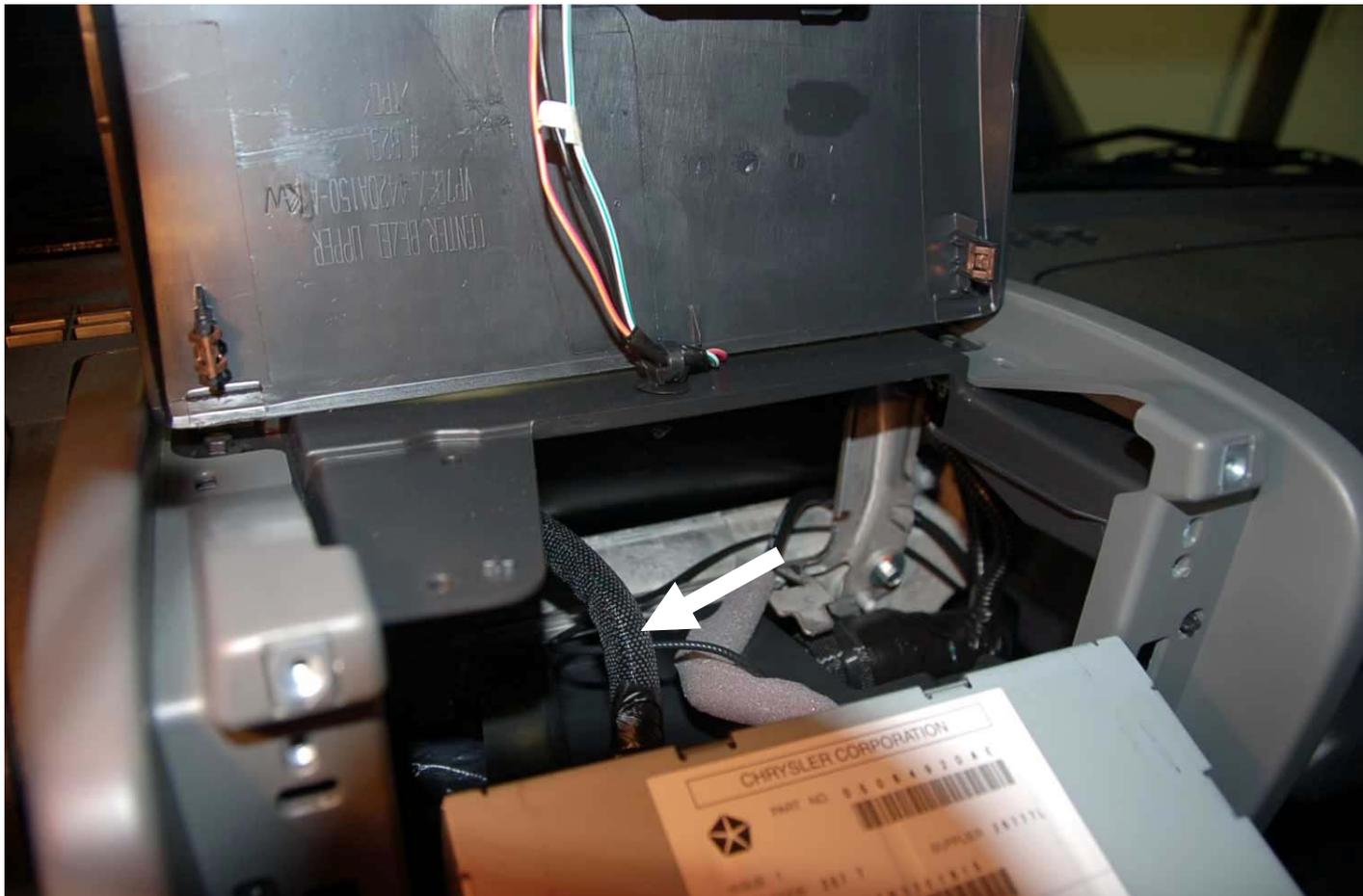
Pull the radio forward until you can reach the power/data cable. You need to press the tab on the bottom of the connector for it to release.
