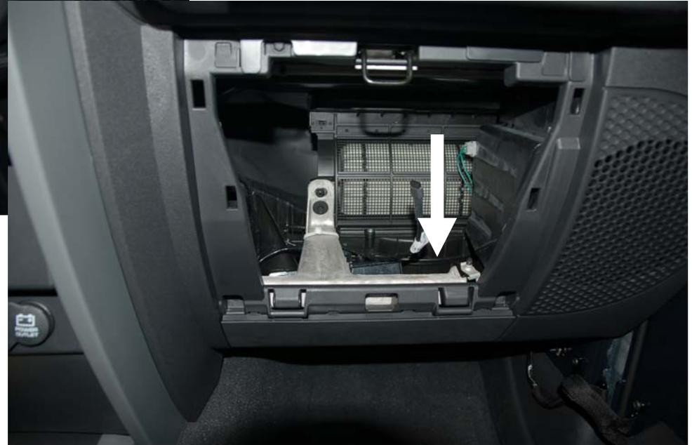
Plug the module in and place under the metal frame. Keep wires from sharp metal.
