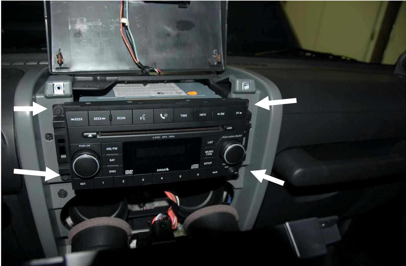
Remove 4 (7mm) radio screws.
