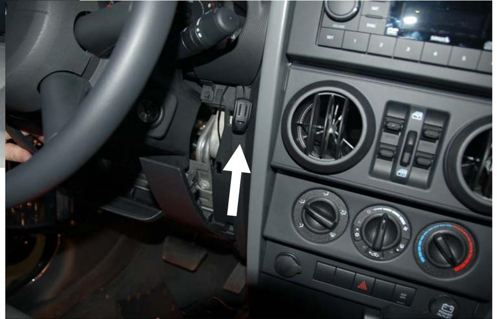
Remove cover under steering wheel from top. Thread microphone into area away from adjustable steering wheel, ignition switch, and heater vents. I haven't completely decided on the final place yet but this area is away from noise that might cause problems with Uconnect.
