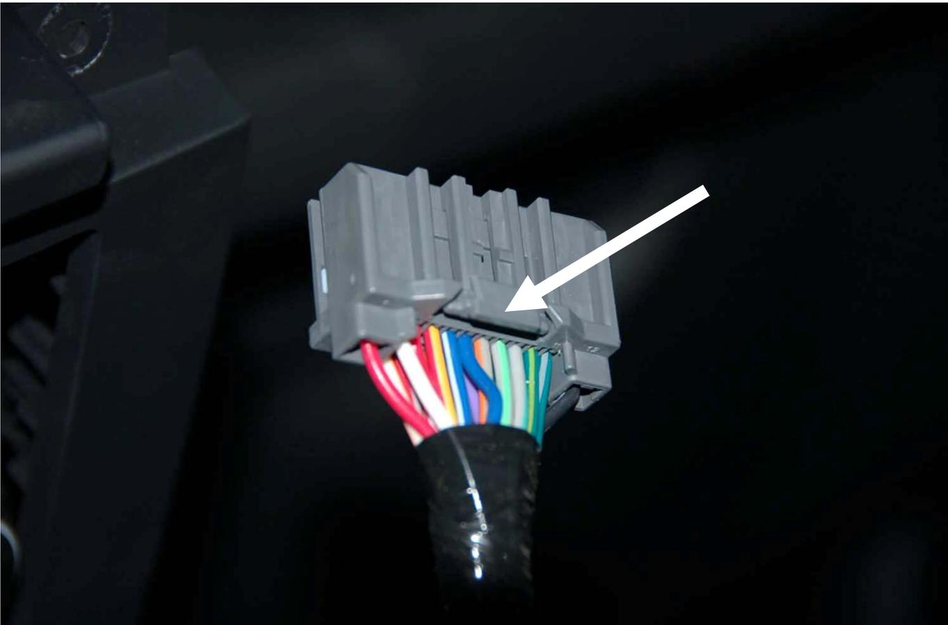
This is the tab on the underside of the connector you want to press in.
