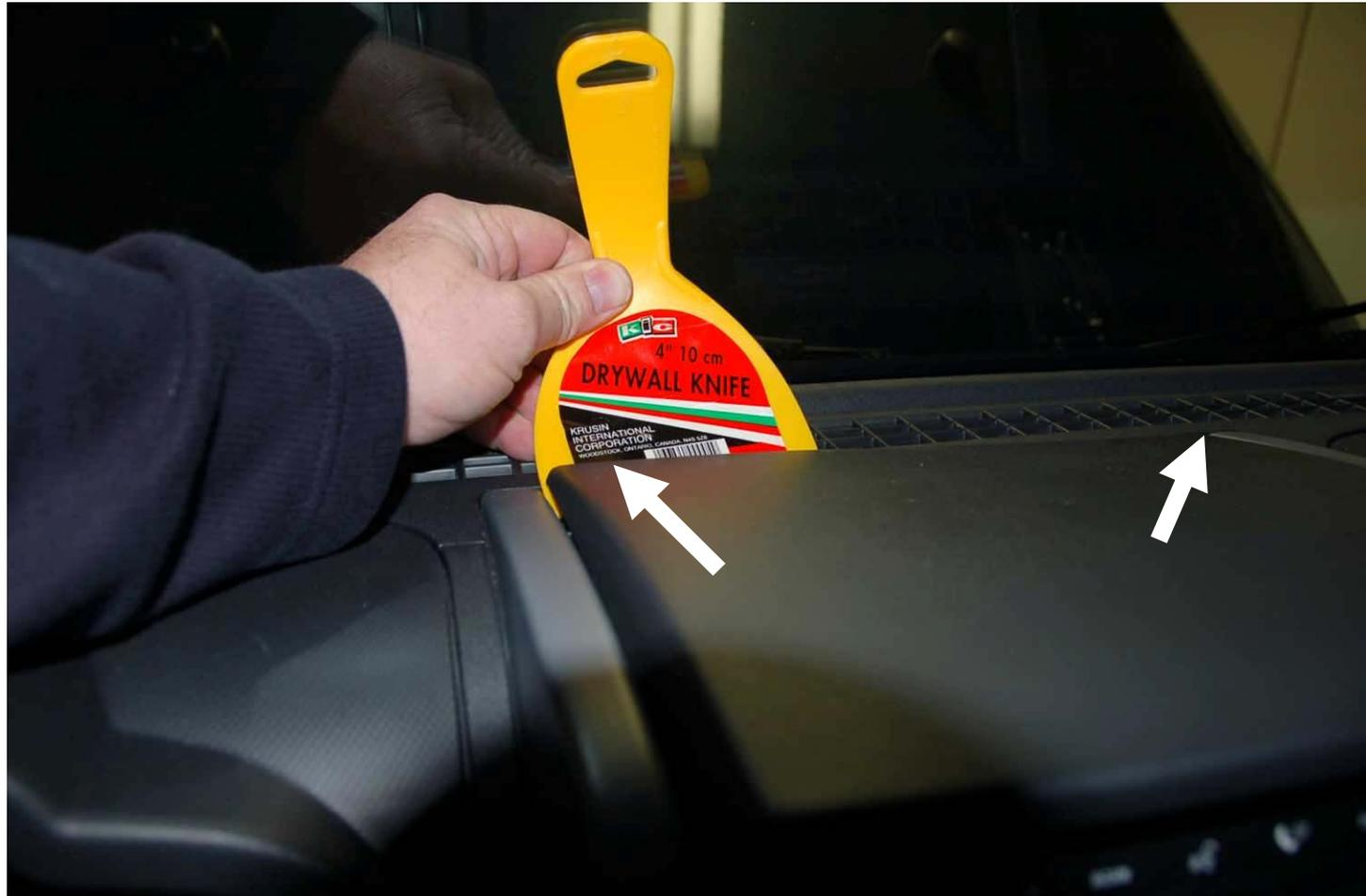
There are two clips to remove, pry under corners not center.
