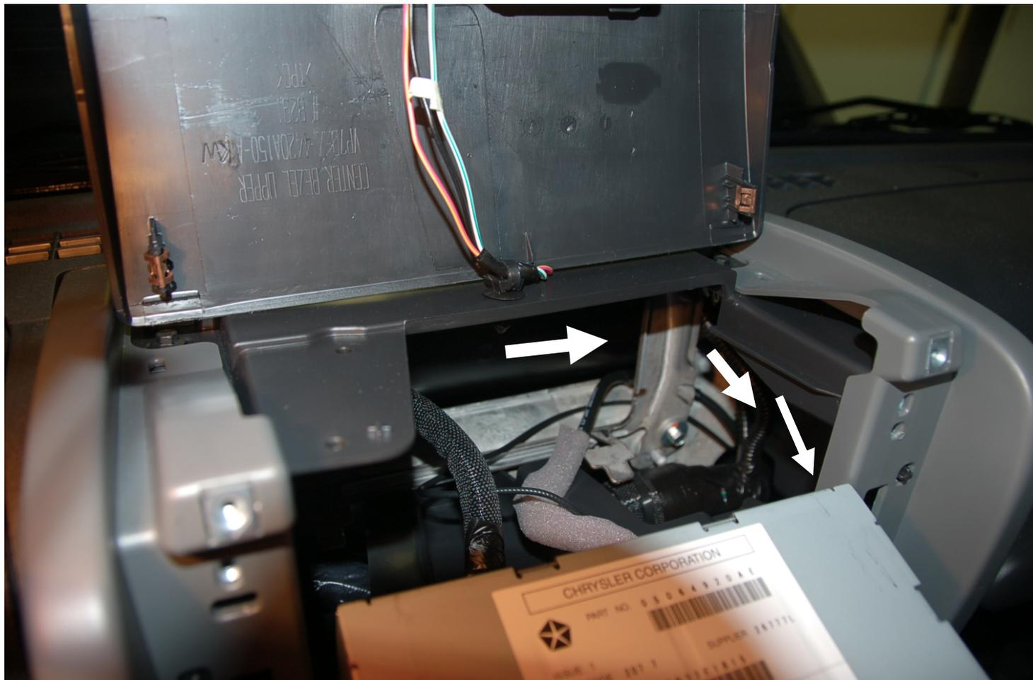
The Y cable is not very flexible and there isn't a lot of room behind the radio. Be patient and gently mold the cable into the space behind the radio. The module cable end must go behind the metal frame and down to glove box. (See arrows) It will fit! Re-install 4 (7mm) screws in radio when cable is routed.
