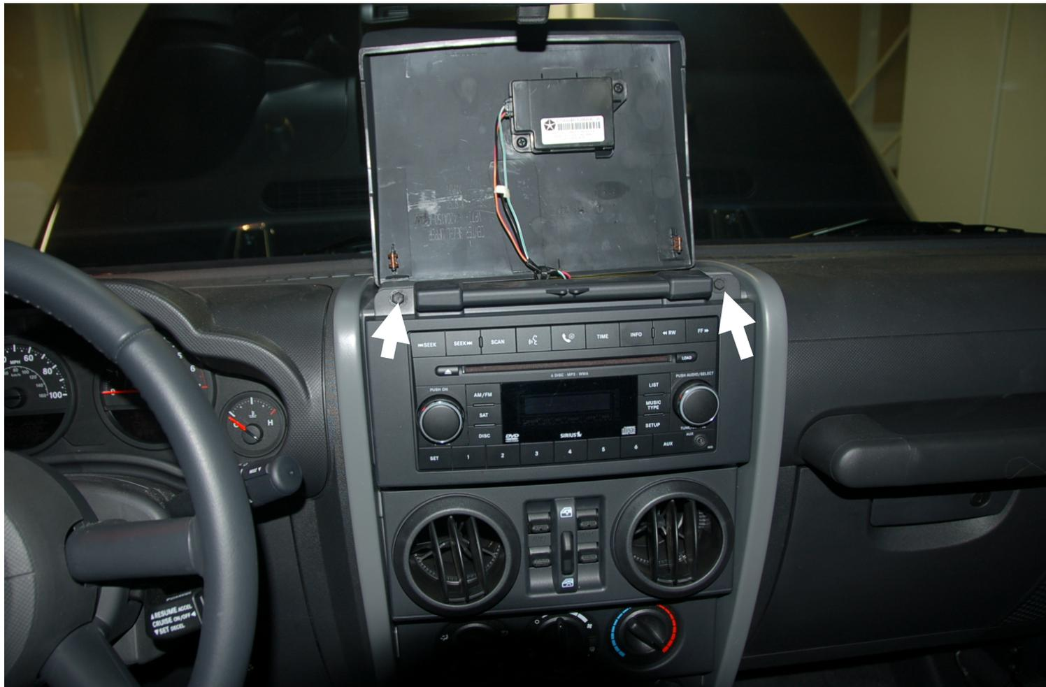
Rest cover on top. Remove 2 (7mm) screws for front bezel.
