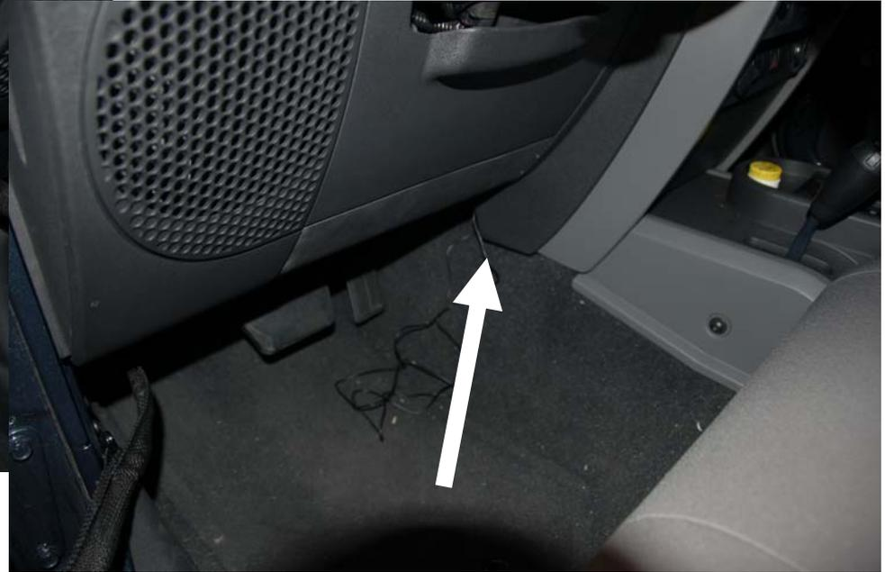
Plug in microphone cable and run under glove box, under center console to drivers side.
