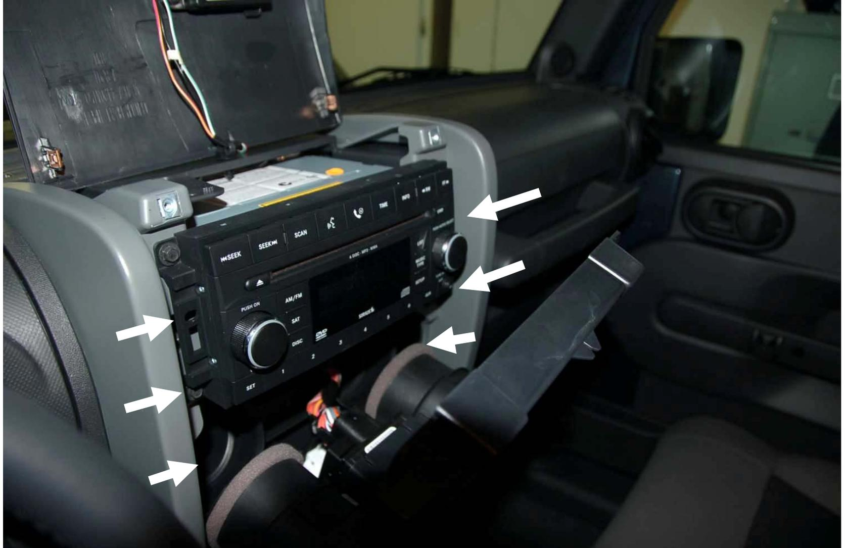
Carefully, gently, and slowly remove front bezel. There are clips on each side to release. 2 on each side of the radio and vents. The entire bezel does not need to come off. Only far enough to remove the radio. About 8 inches.
