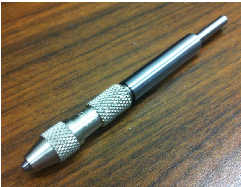
Figure 4.11: Assembled Chuck & Shaft
