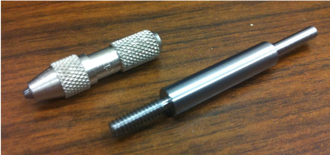
Figure 4.10: Disassembled Chuck & Shaft
