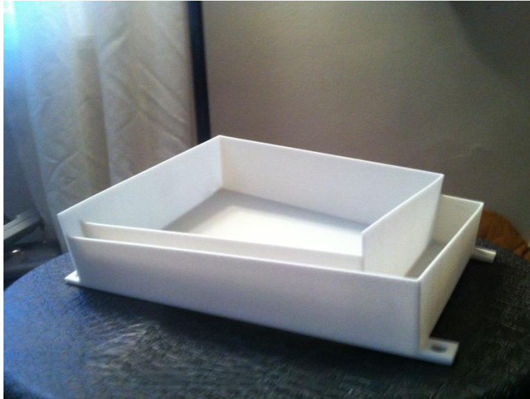
Figure 4.7: Warped Bath Prototype (Isometric View)
