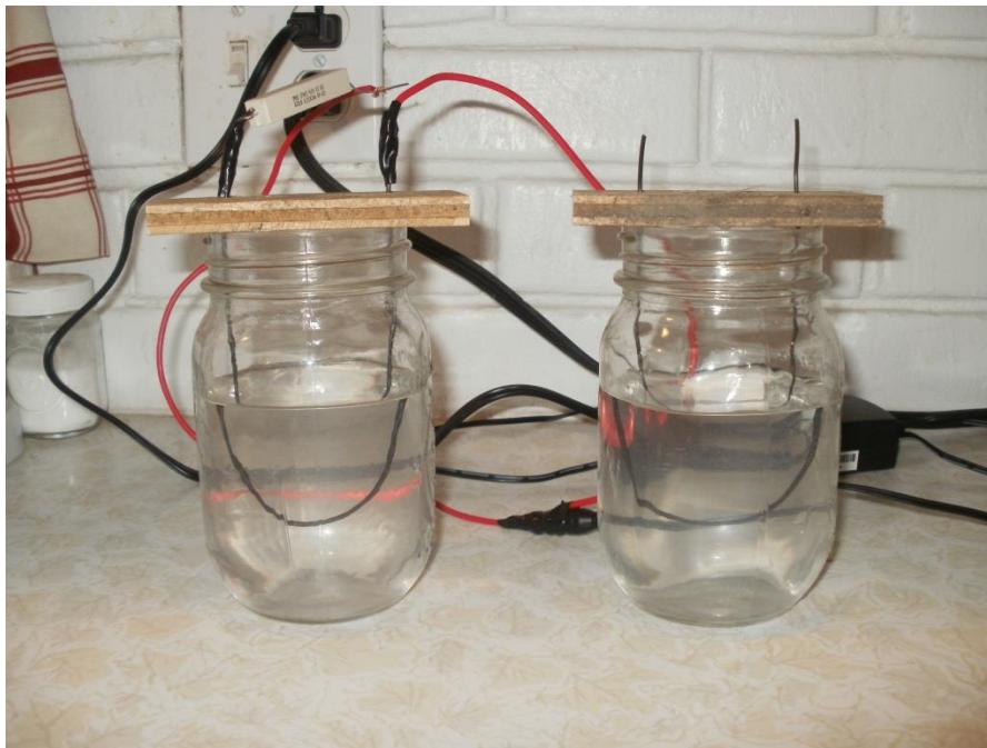
Figure 5.1: Corrosion Resistance Test Under Constant Current Conditions
