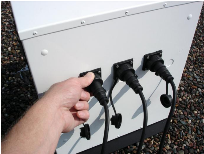
Figure 40: Connect Power from the Solar Cell Power System to the Environmental Enclosure
