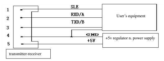
Remarks: To avoid to connect the interface reversely and can not communicate, please check and assure the voltage of 2 and 3 pin is existing by using multimeter. If there is one pin that has the voltage, another has not voltage, which means the interface is connected reversely, pls. Change the connection wires between pin 2 and 3.
