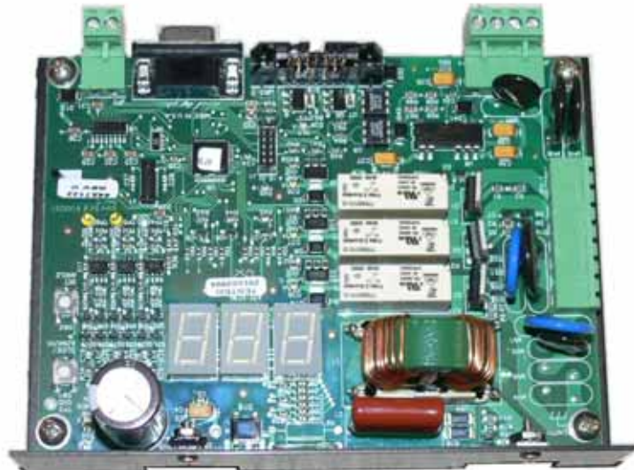
Figure 9: Light Unit Control Board Indicators and Test Points
