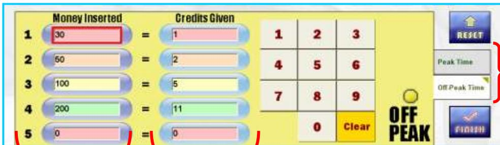
This allows the user to set the type of money customers can put in. The values in fig. 2.8 are preset but can be changed if the user wishes to by using the Numerical keypad. Each number denotes a unit of currency, for example 100 = £1.00, 20 = £0.20 and so forth.
