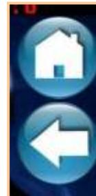
These two buttons allow the user to navigate through the screens to either back to the Main Menu (home icon) or back to the previous screen (back arrow icon). These two buttons will perform the same functions on any screen and so will only be mentioned in this section of the manual.
