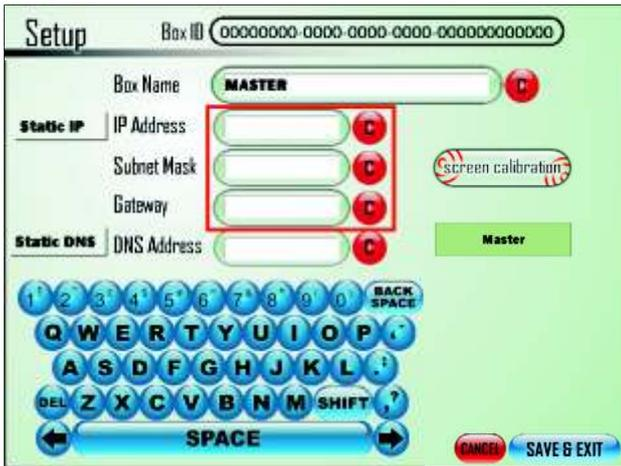
The Screen above shows what happens when the user presses the DHCP IP Address Button. Here, highlighted in the red box are the Active Address fields, to allow allows the user to enter a Static IP Address and settings. Notice also how the DHCP IP Button has changed to read Static IP. Pressing the same button again greys out the fields and returns to the automatic DHCP IP Address settings.
