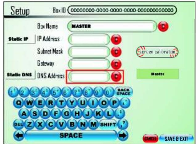
The Screen shot above shows what happens when the user presses the DHCP DNS Address Button. It follows exactly the same principle as the DHCP IP Address Button, except that it only activates one field (highlighted in red). Pressing the same button again returns to the automatic DHCP DNS Address settings button.
