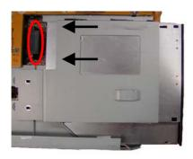
Step 3: Fix the CD-ROM and the base on the rack with 2 screws.
