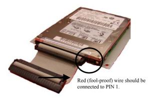
Step 2: Fix the hard drive with its rack on the four posts and connect the ribbon cable to the IDE connector (J1).
