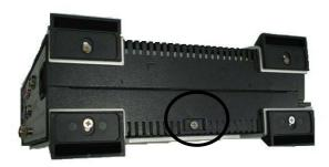
Step 2: Grasp the handle on the panel and pull out the case.
