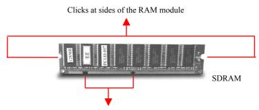
Align the fool-proof clicks on the bottom of the RAM module to the socket, and the locks on the socket should securely lock on the clicks at sides of the module as shown in the above picture.
