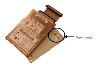
(Attention! Make sure that the red (fool-proof) wire on the ribbon cable should be connected to PIN 1 of the hard drive as shown below.)
