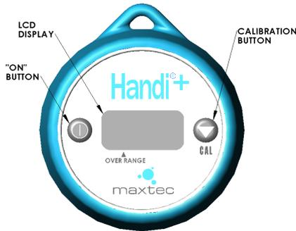
**LCD Display:** A 3-digit display provides a direct readout of oxygen concentration in the range of 0 - 100%. The display is blank when the Handi<sup>®</sup>+ enters its Sleep (power off) mode. The Handi<sup>®</sup>+ will automatically enter the Sleep mode after approximately 1.3 minutes from the last time the ON button was pressed.
