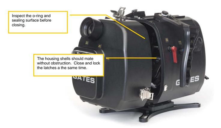
✓ Carefully inspect the parting line between front and rear housing. If this line is not even all the way around, remove the back and determine the reason. (O-ring out of place, hand strap interference, etc.) Failure To Do This May Result In A Wet Camera!
