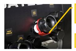
Position the Lockout Collar here to prevent contact with the manual iris ring of the camera.
