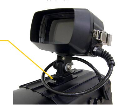
Connect and secure the video connection. The 6 pin HD connector is shown. Other monitors may use single pin SD connector.
