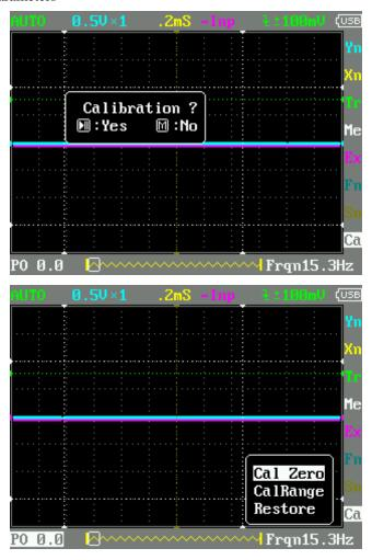
Oscilloscope Calibration: Press
