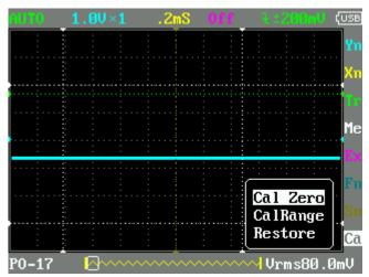
3. Select "Cal Zero" option, by "O" or "O "change the cursor blink in the parameter value is adjusted for PO 0.0 "Zero calibration line, line with the arrow to a level.
