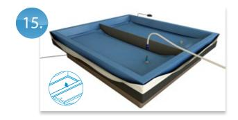
Smoothen the water mattress thoroughly, removing all folds. Make sure that the 4 corners snugly fit the corners of the foam borders.
