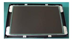
Tear off the outer layers of dust-proof strips for about 3 or 4mm
