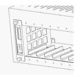
**Connecting to Power (Power Supply)** To install a power supply to this chassis, please slide the power supply to the chassis and fasten the hand screw clockwise to the chassis.
