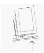
Step 4: Press the converter gently and push it to the left side to make sure it is fitted into the bay cover.
