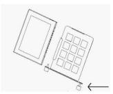
Step 3: Carefully locate the converter in the bay cover.
