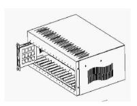
Step 6: Fasten the hand screw clockwise by hand to make sure it is firmly fitted into this chassis.
