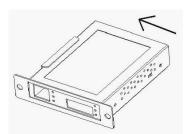
Step 5: Slide the bay cover with the converter into the slot of this chassis until it is fully fitted.
