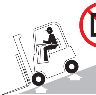
No parking on ramp
