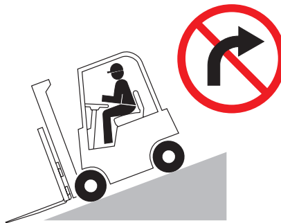
No turning on ramp
