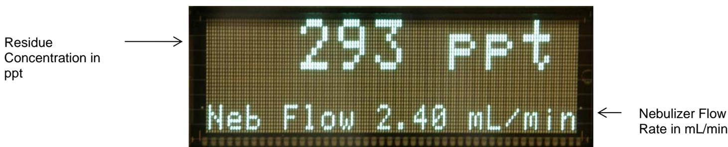
The NRM 8000 collects residue concentration data in  $\#/cm^3$  every tenth of a second. This raw particle count data is accumulated and used to calculate and report residue concentration as parts per trillion (ppt). The displayed concentrations are based on the most recent five seconds of data and are updated each second. The displayed values range from 0 to 60,000 ppt.
