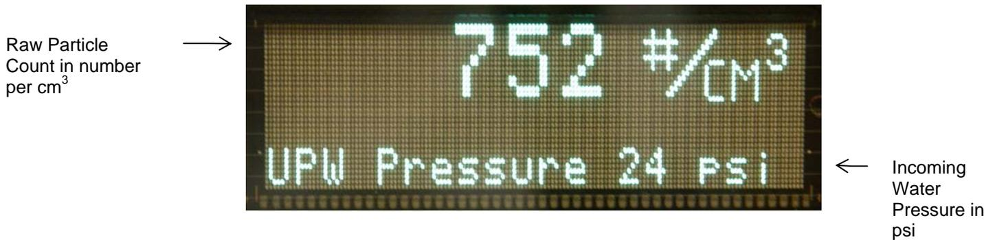
The raw particle count is a count of the number of residue particles formed as each nebulizer droplet is dried. It is not a particle count of particles present in the water (as measured by a conventional liquid-borne particle counter).
