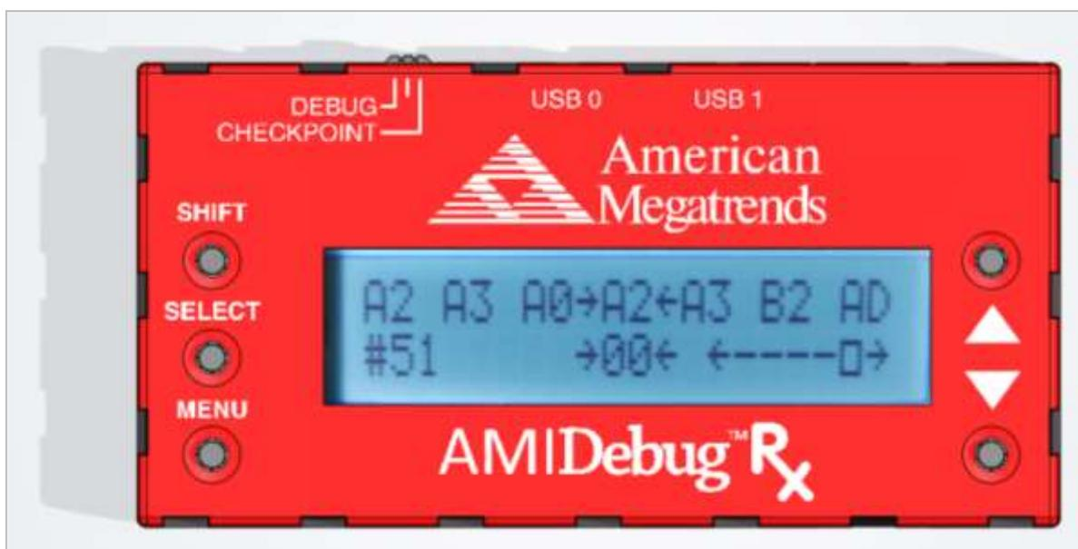
USB0 LED – indicates connection (ON) & activity (BLINK) for USB CONNECTOR 0
