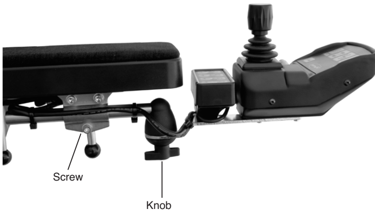
Length adjustment screw
