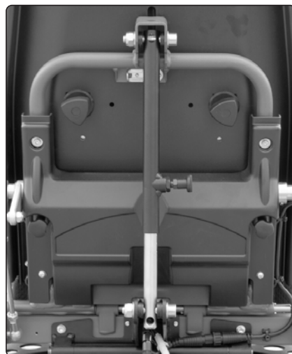
Manual locking tube for backrest recline.
