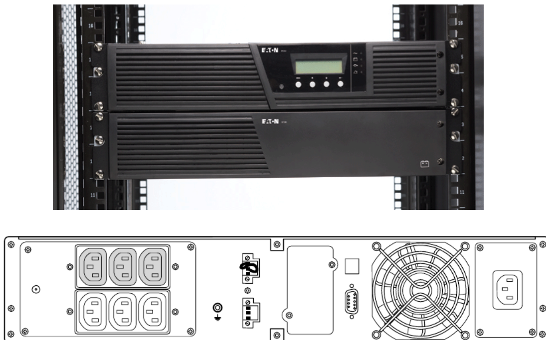
Figure 4.2: (top) UPS system selected for Supercam electronics is a 2U rackmount system with 230VAC capability and a remote, managed interface. Only the top 2U unit will be used; the bottom module in the figure is an add-on battery module for extended runtime. (bottom) The back face shows the connectors needed to interface with the APEX power system. Schuko to IEC cable adapters are baselined.
