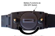
Rotate Clockwise to Turn Collar ON
