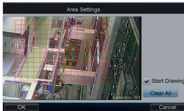
6. Click **Start Drawing**, and then use the mouse to click two points on the live view screen to draw area for motion detection.
