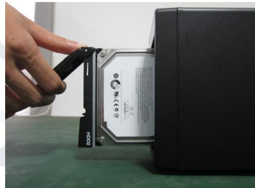
2. Put the HDD to the HDD box at the front.
