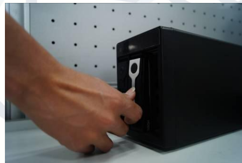
4. Put the knob back after you insert the HDD to the SATA board.
