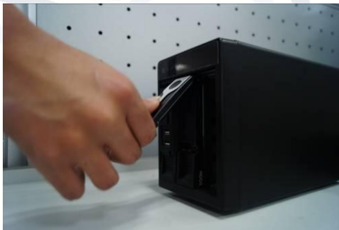
3. Pull the HDD knob up when you put the HDD into the box in case the knob buckle may strike the front panel.
