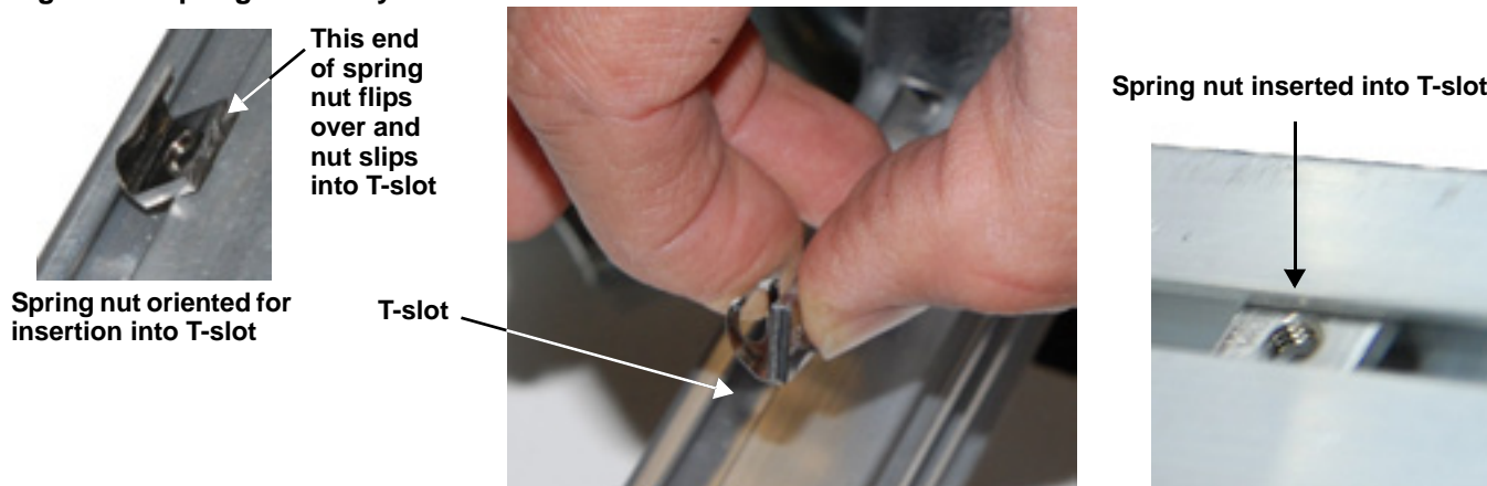
Figure 4 Spring nut ready for insertion
