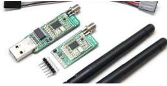
Figure 3.5: Telemetry Radio from 3DR Robotics.
