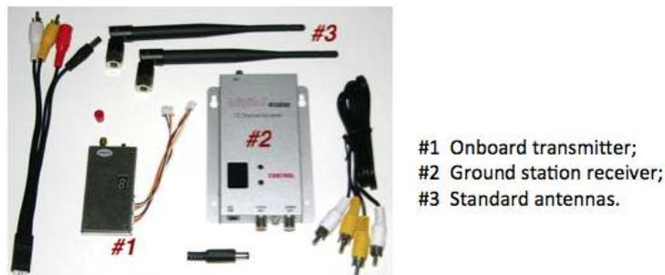
Figure 4.3: Video system developed by Partom.
