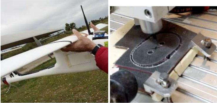
(a) Test for Thrust. (b) Final Result for the support of the motor.
