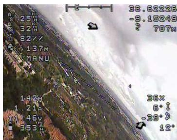
Figure 7.6: Banking of  $-39^\circ$  with no image distortion.
