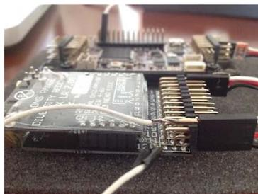
Figure 5.4: APM reads RSSI from Ch12 to channel A1.
