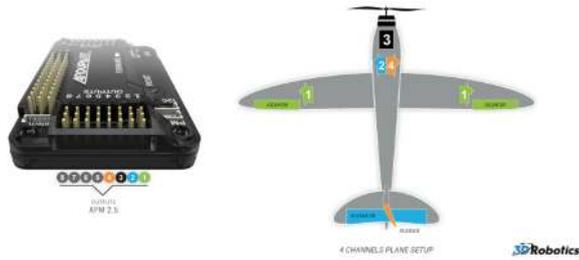
Figure 5.1: 4 Channels plane setup [63].
