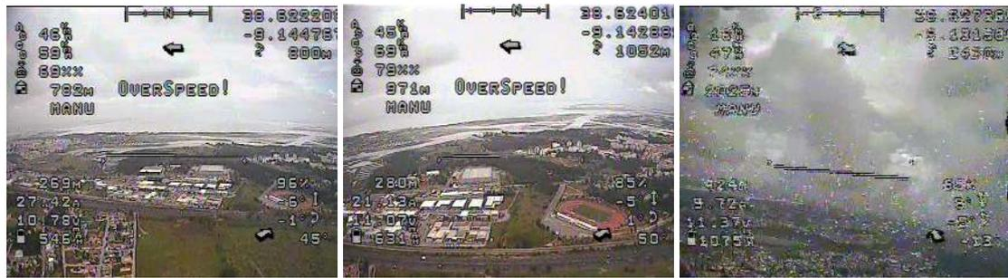
(a) Effect of reorienting the Helical antenna towards the UAV (#3). (b) Making use of the camera gimbal to do a terrain recognition (#4). (c) Video loss at 2.03 km from the GCS (#5).
