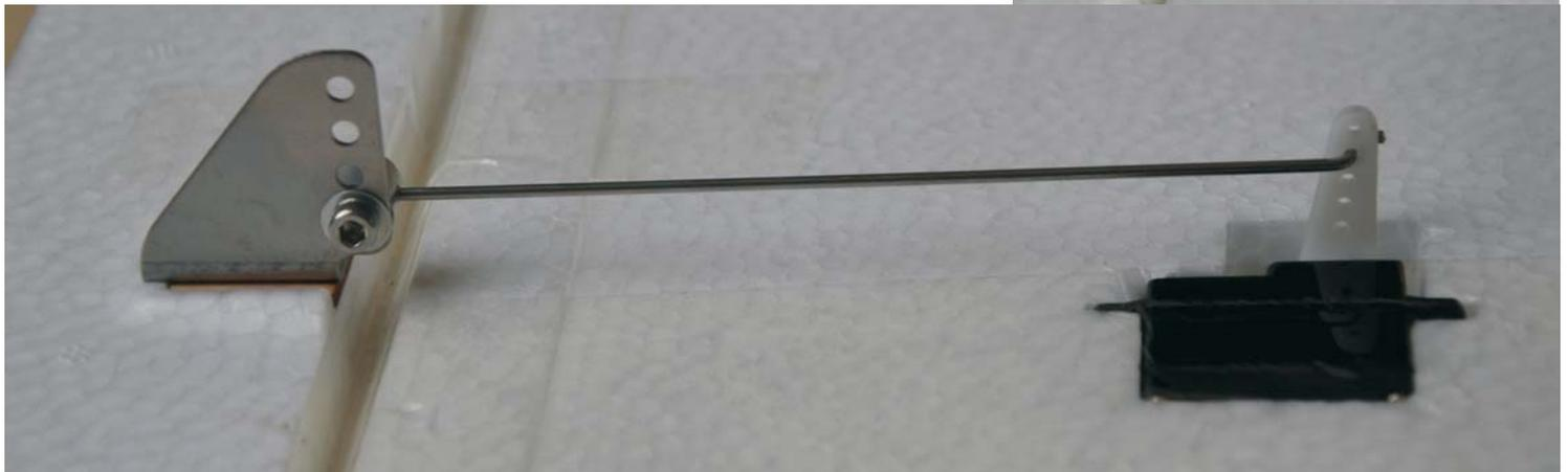
Vertical stabilizer (Rudder) \_ Servo&Servo horn installation
