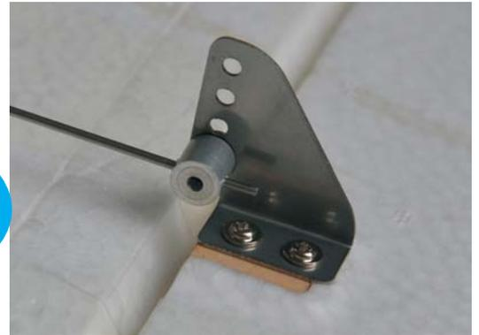
Main wing Aileron Servo&Servo horn installation
