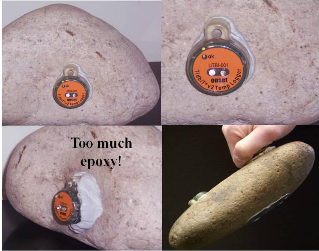
Photo 7. Temperature sensor attached to rock surface with the Fox epoxy in a laboratory setting. Once the epoxy fully sets in ~24 hours, the sensors are firmly attached to the rock surface. Lower left panel demonstrates applying too much epoxy to attach the sensor, which would prohibit use of the underwater shuttle. Lower right panel shows a 5 pound rock held aloft by the sensor.
