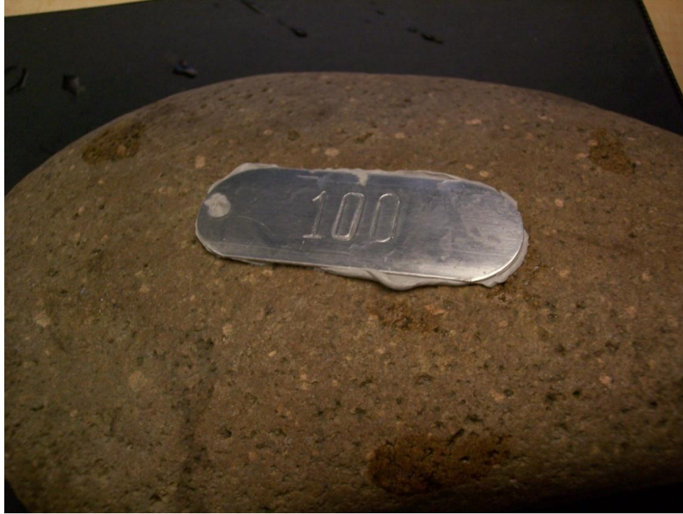
Photo 11. Metal forestry tag attached to the top of a rock with the Fox epoxy to monument the location of a stream temperature sensor.
