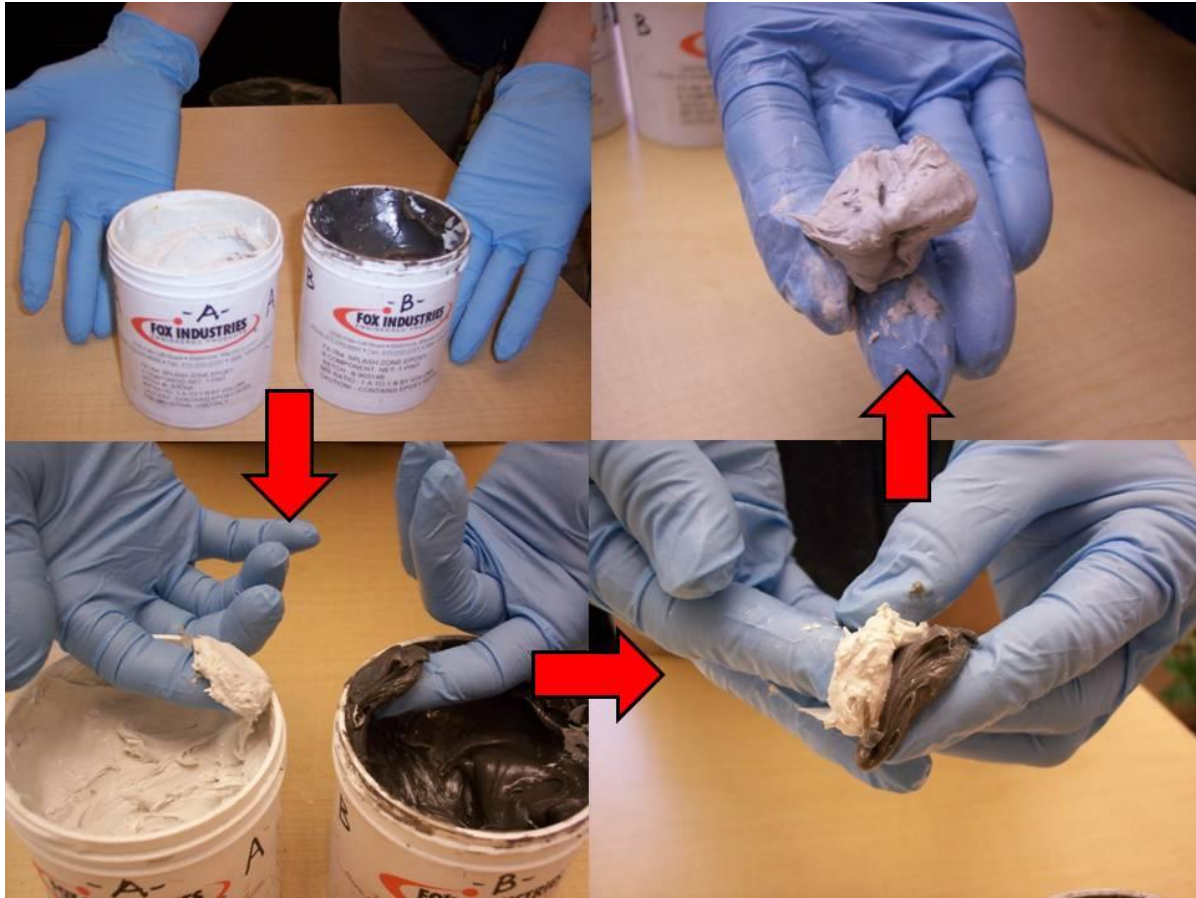
Photo 5. Preparing the Fox epoxy for use involves extracting equal amounts of each component and mixing together for one minute until the color is uniform throughout. Fingers should be wetted before and during handling the epoxy to minimize messiness.
