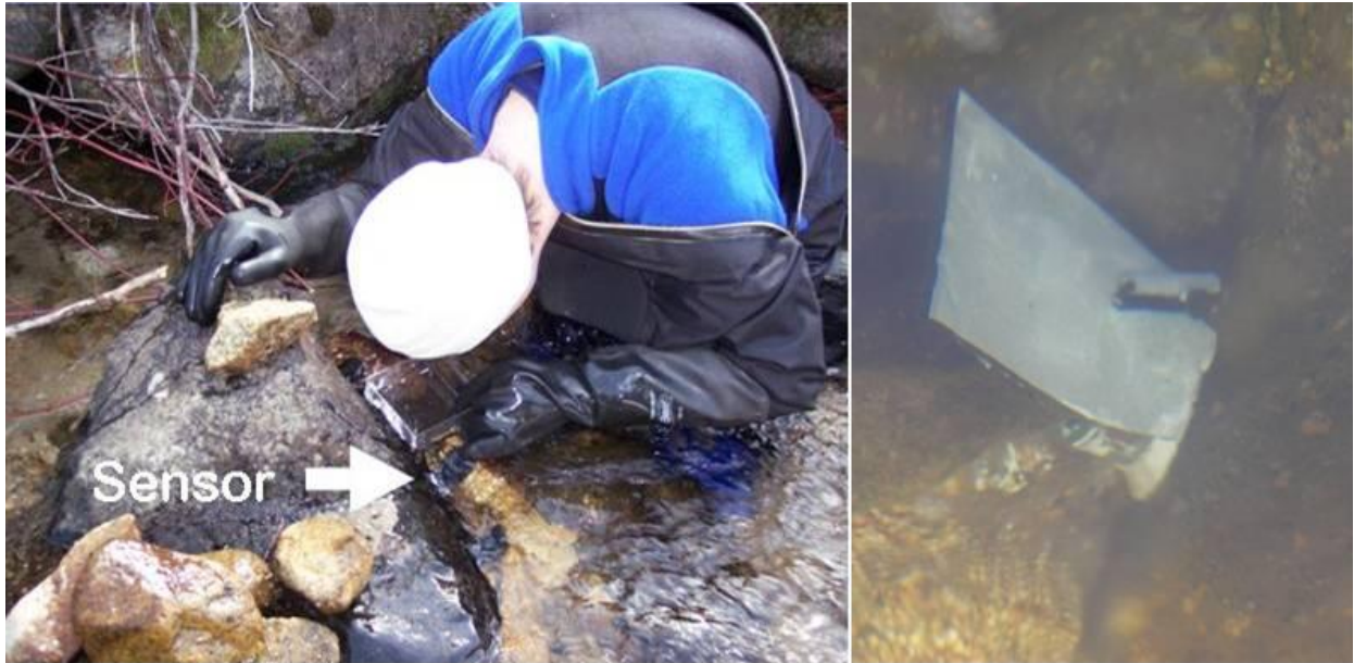
Photo 9. Inspecting a temperature sensor attached to a rock surface using a viewing box in the field.
