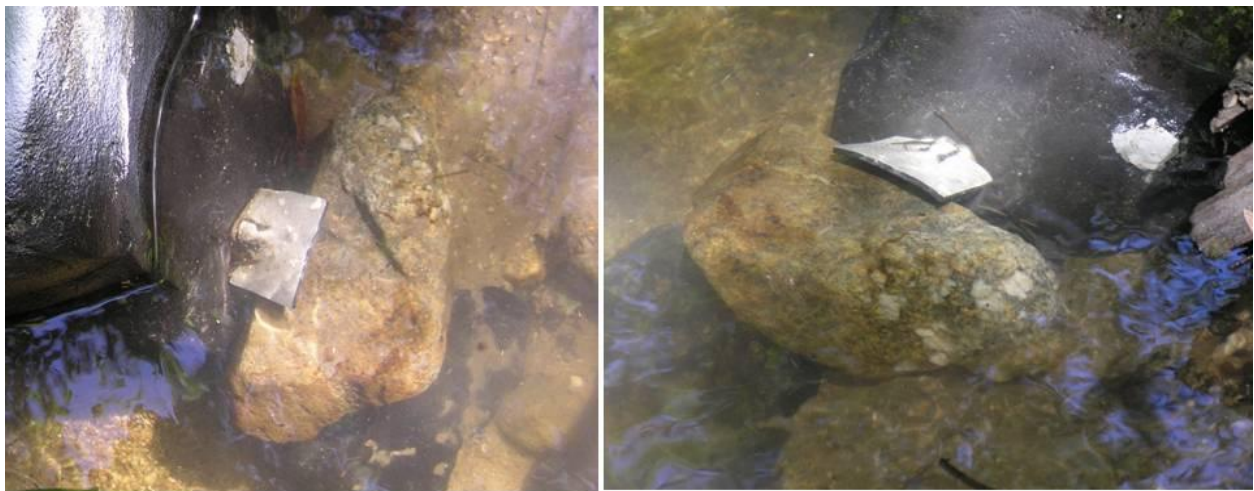
Photo 10. Temperature sensors glued to rocks in mountain streams. Notice the rocks propped against the front of the sensors to hold them in place while the epoxy sets. Smaller prop rocks than those shown are typically used because only a small amount of pressure is needed.
