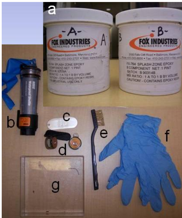
Photo 1. Equipment needed to permanently install temperature sensors in streams using underwater epoxy includes: (a) FX-764 from Fox Industries, (b) underwater data shuttle (if data are to be retrieved in situ ), (c) metal forestry tree tag, (d) temperature sensors, (e) wire brush, (f) rubber gloves, and (g) plastic viewing box.
