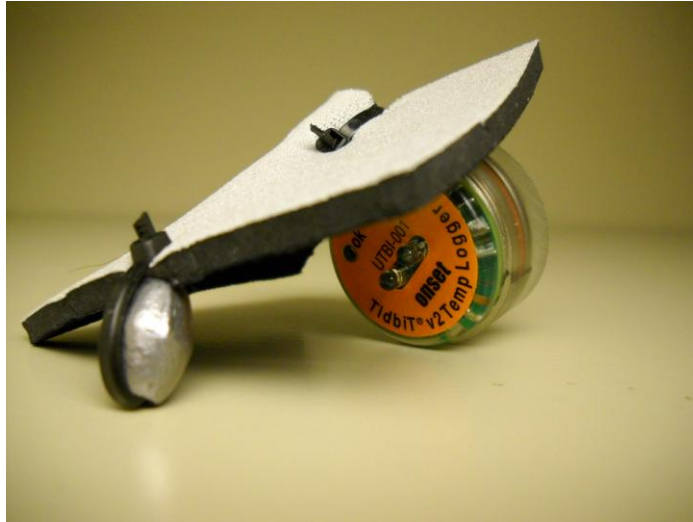
Photo 3. A small lead weight attached to the front of the solar shield causes the flap to hang in front of the sensor (providing the best possible protection against direct sunlight) and prevents the shield from being lifted by turbulent flows.
