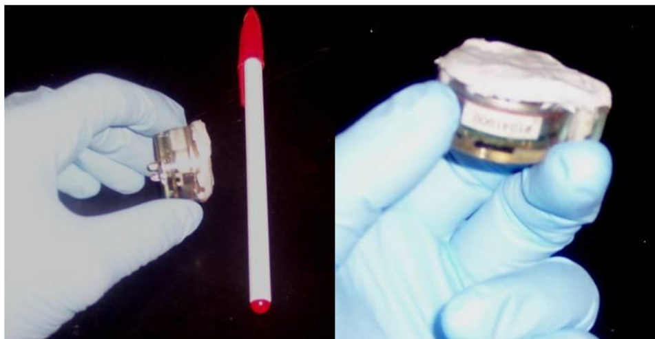
Photo 6. Fox epoxy applied to the back of a temperature sensor ready for deployment. Enough epoxy should be applied that it can cover the surface of the sensor to a depth of approximately 1/8 inch.
