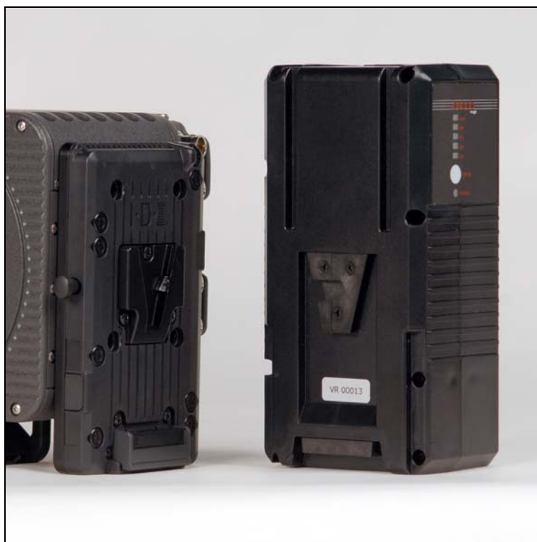
Figure 8: ALEXA with BAB-V and V-Mount battery
