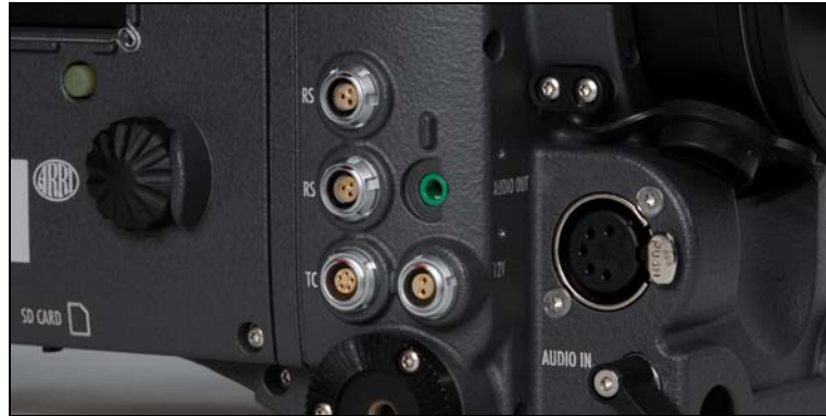
Figure 10: 24 V outputs (RS) and 12 V output
