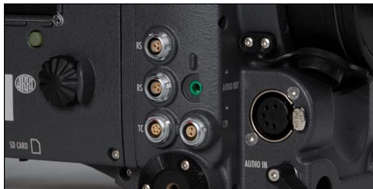
Figure 24: Connectors on right side
