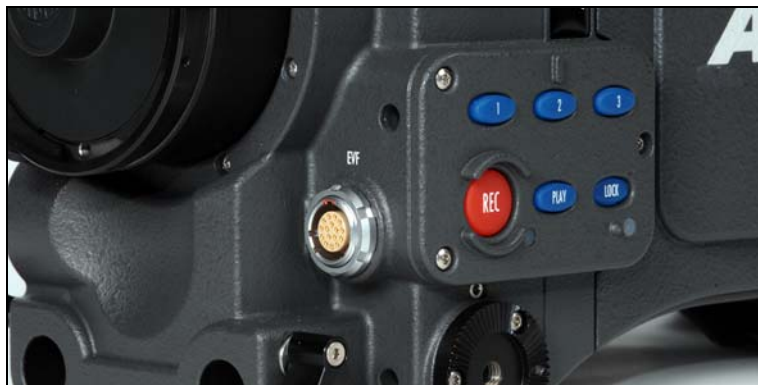
Figure 26: Camera front connector
