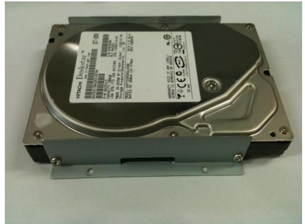
2. Install the mounting bracket on the HDD.
