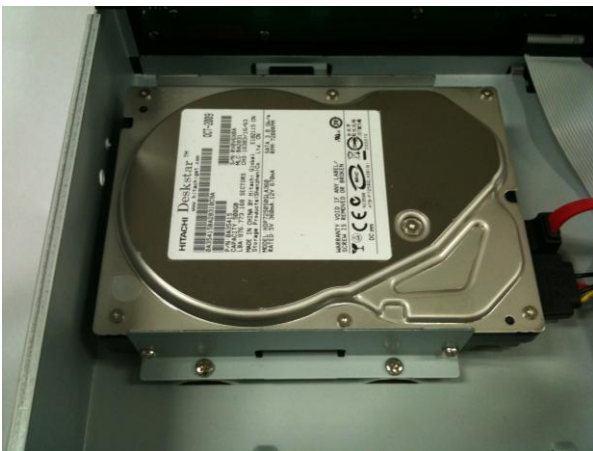
3. Installation HDD and Bracket onto base case (Inside)
