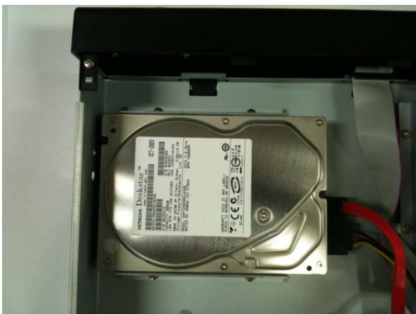
5. Connect the Data Power cable to the HDD.
