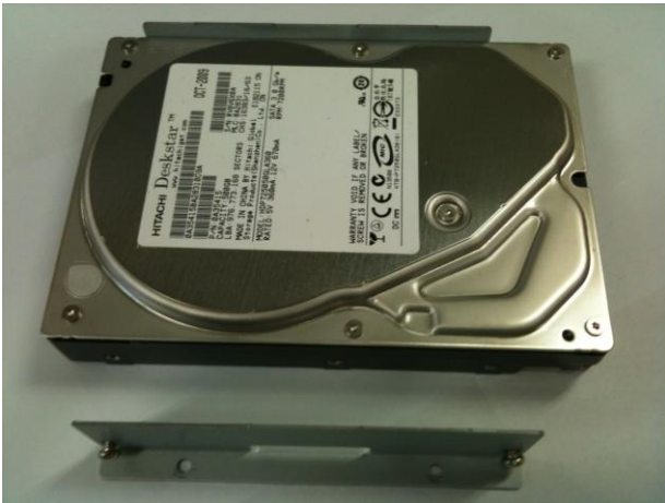
1. Before installing bracket and screws onto the HDD.
