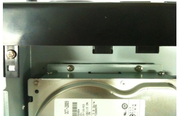
4. Installation HDD and Bracket onto base case (Outside)
