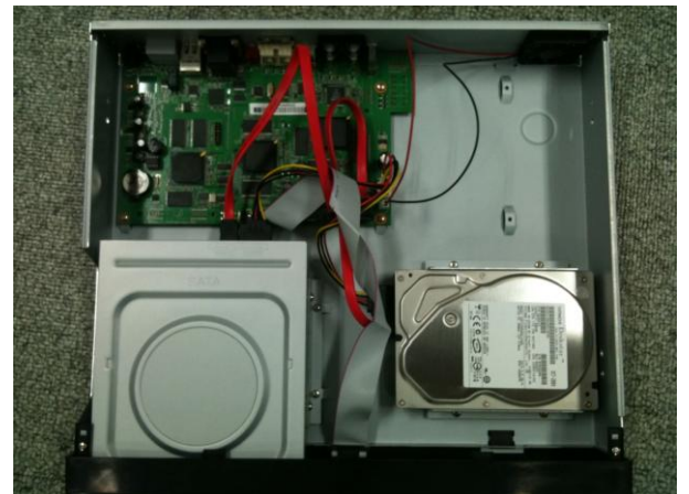
6. Installed HDD and DVD-RW.
