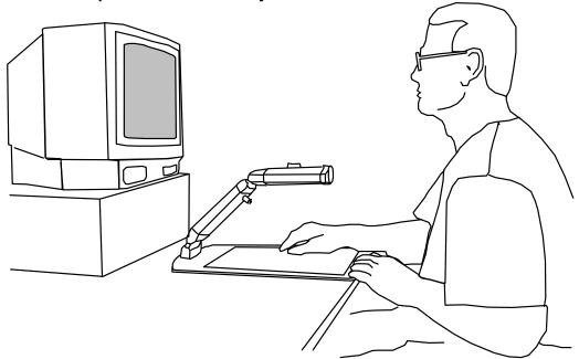
Place the material you wish to read on the reading table and adjust the focus knob until a sharp image is obtained. Adjust the magnification as described above to suit and re-focus if necessary. Ensure the camera head is horizontal for optimum image quality.
