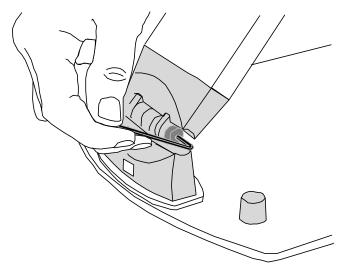
If the hinges loosen with use they can be tightened with the Allen key provided. To do this, pull off the caps covering the hinge screws and insert the Allen key into the screw head. Turn each screw clockwise about a quarter turn . do not over-tighten. Replace the caps. Loosening of the hinges is not covered under the terms of warranty; it is a user-maintenance issue.
