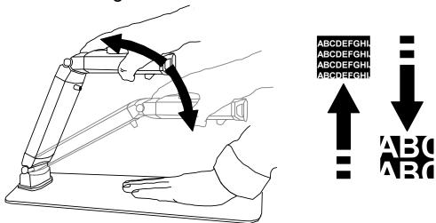
Lower the camera for higher magnification; raise it to reduce the magnification.
