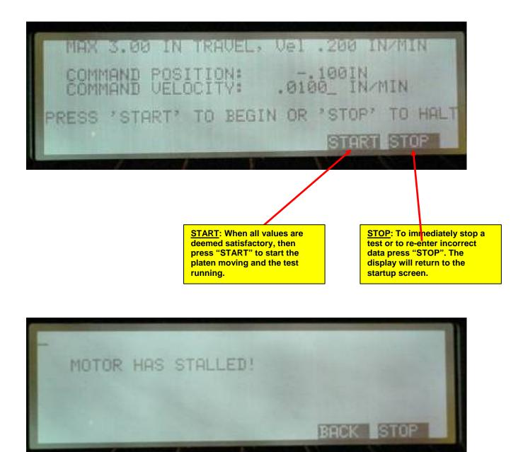
The motor stall screen is displayed when the Load Frame has reached its operating limit or, in the FAST UP mode only, a reduced limit. This reduced limit in FAST UP is done to help protect attached instruments in case of operator error.
