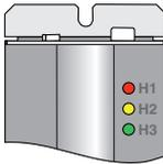
At the top right of the positioning drive there are three status LEDs colored red (H1), yellow (H2) and green (H3).
