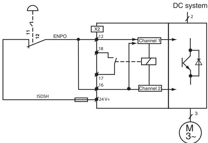
Figure 3.12 Connection example with Emergency Off button
