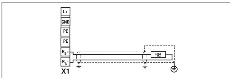
Figure 3.11 Braking resistor connection
