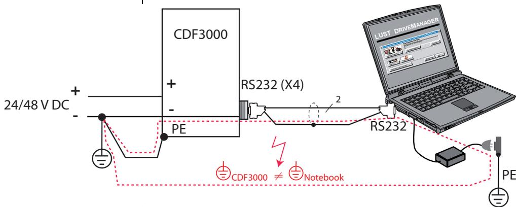
Figure 3.9 Serial interface connection
