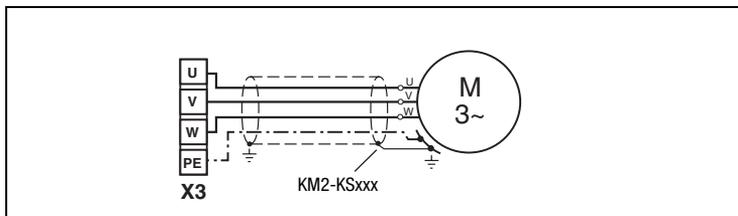
Figure 3.5 Connection of motor
