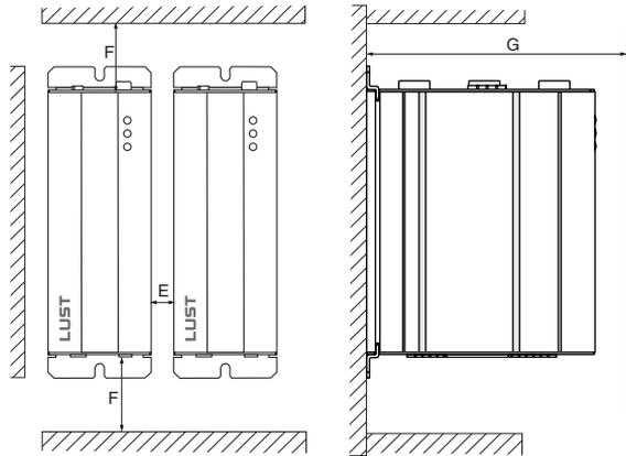
Figure 2.1 Mounting clearances (see Table 2.1)
