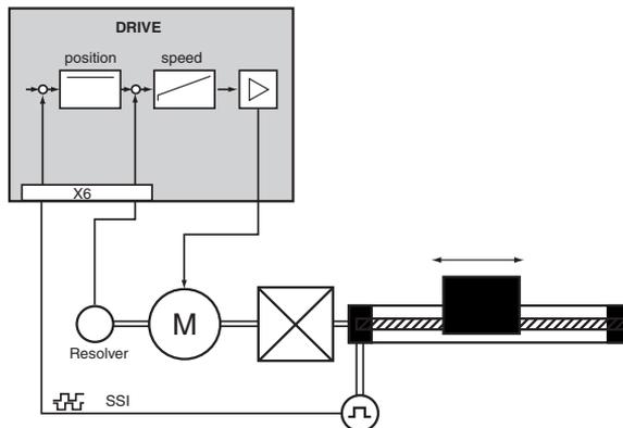
Figure 3.7 Drive with two measuring systems
