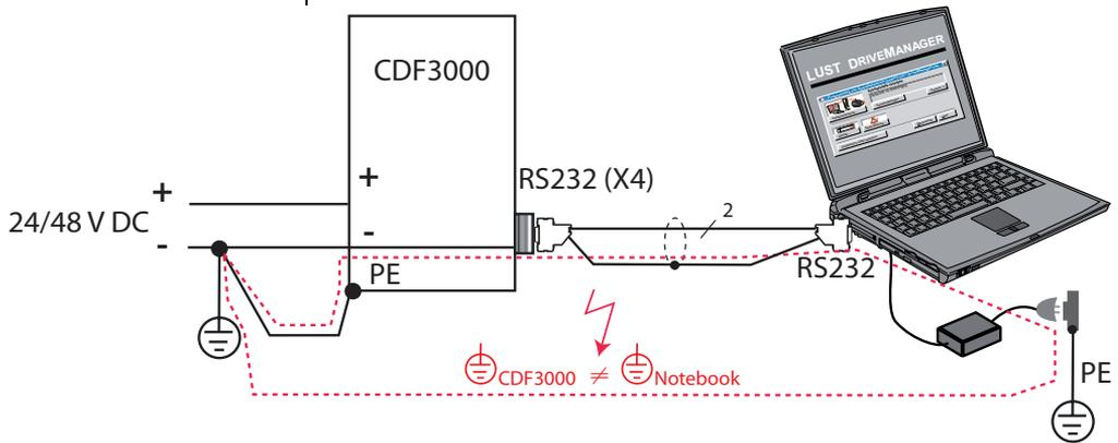
Figure 4.3 Serial interface connection
