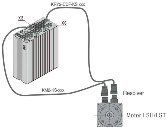
Figure 3.6 Matching motor/encoder cable
