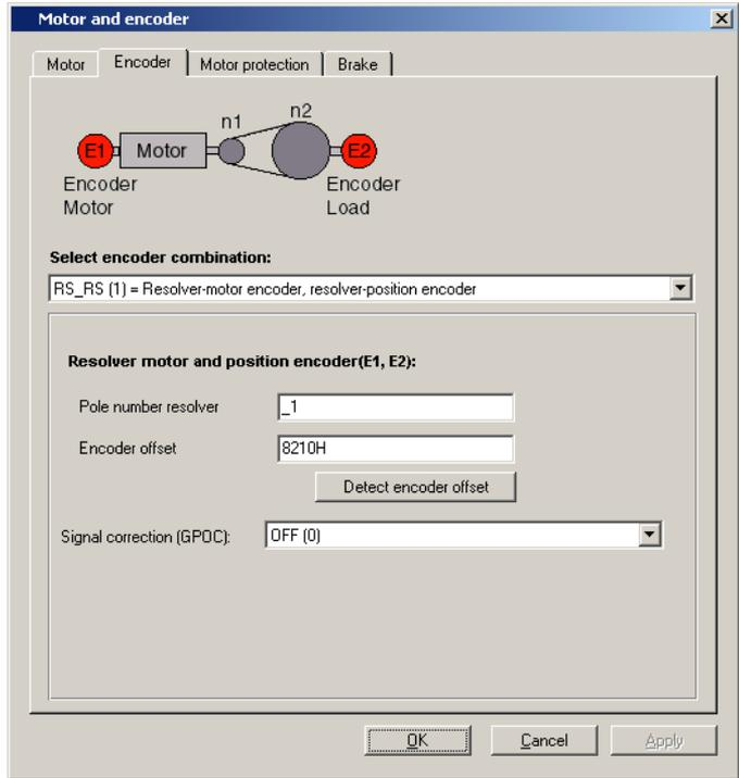
Figure 4.5 Encoder configuration
