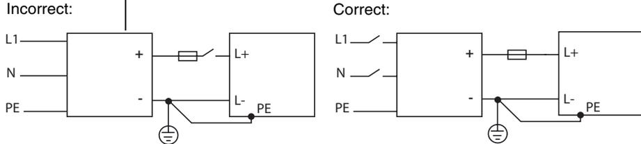
Figure 3.4 Connection of supply voltage
