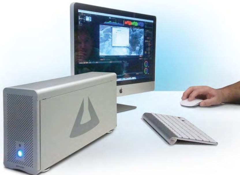
**Note:** ExpressBox 3T does not have ON/OFF switch. The BLUE LED on the front is an INDICATOR, not a power SWITCH. To turn ON the expansion chassis, connect to a Thunderbolt equipped computer.
