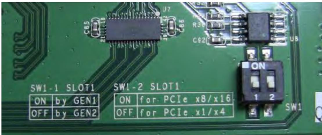
1. If you are installing a X8 . Gen1 PCIe card: set SW1 to ON and SW2 to ON
