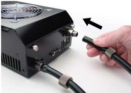
Squeeze the tube while pushing it firmly over the nozzle. Tubing should completely cover the nozzle.
