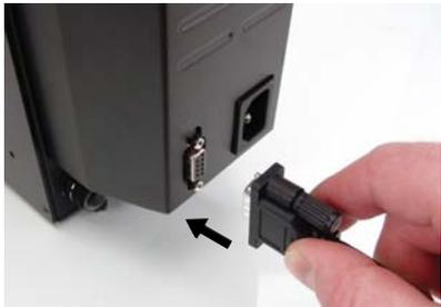
Plug the external 9-pin cable into the cooling system. This plug carries the temperature sensors, extra fan power (optional), power on/off, flow meter signal, and safety signals.
