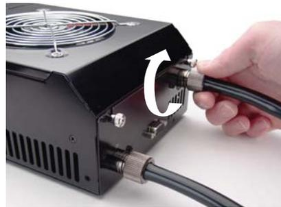
Tighten the connection by sliding the compression fitting down over the nozzle and screwing securely. For hose barbs, use pliers to move it into the proper position.
