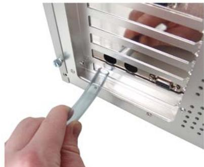
From the rear of the case, carefully feed both ends of the liquid tubing through the Slot Adapter and into the chassis.
