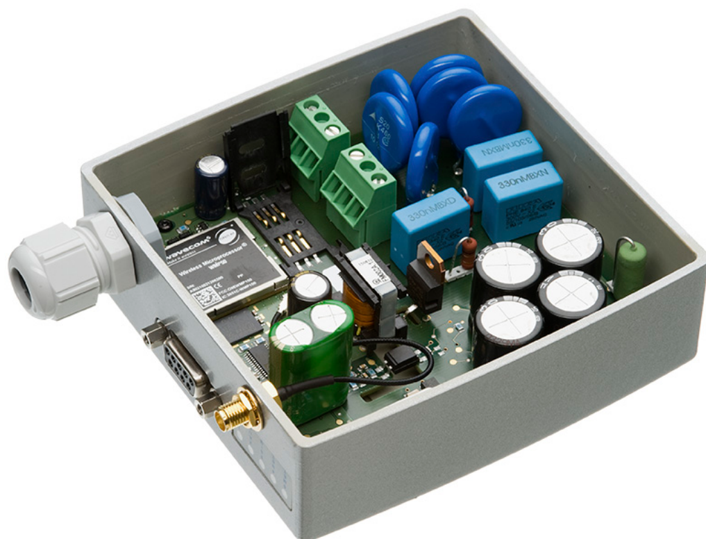
Figure 4. SIM holder open for installing the SIM card
