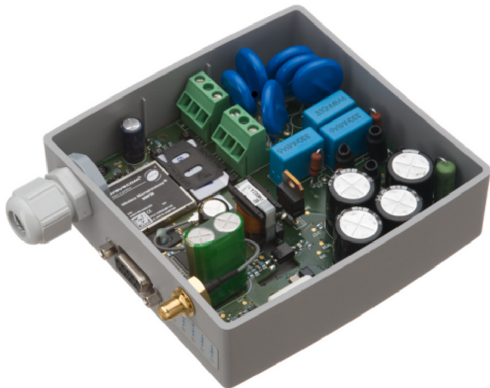
Figure 5. SIM card inserted and SIM holder closed
