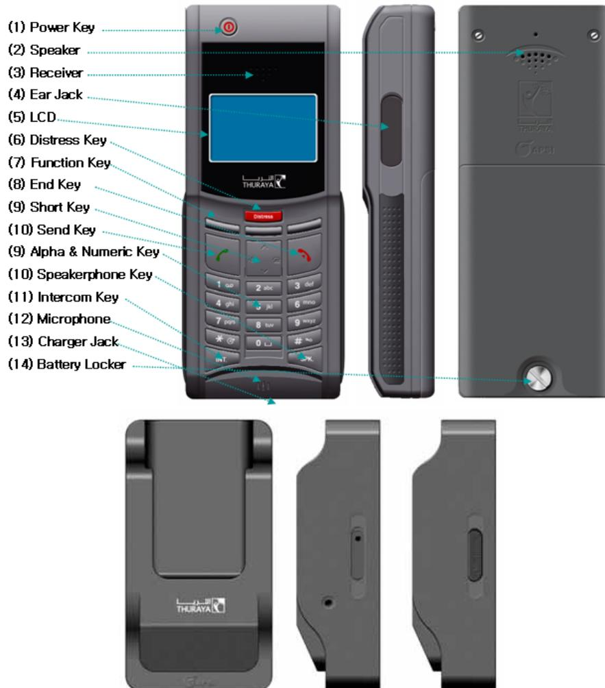
The Handset is the primary interface for the Main Unit. It enables the user to dial numbers, it displays status messages, and it can be used to configure the Main Unit and Handset.
