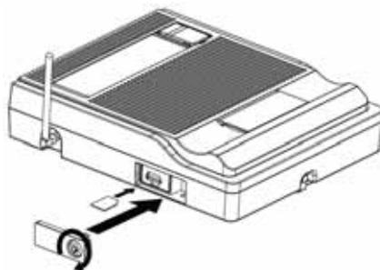
**Note: Turn off the power before inserting or removing the SIM card from the ThurayaMarine.**
