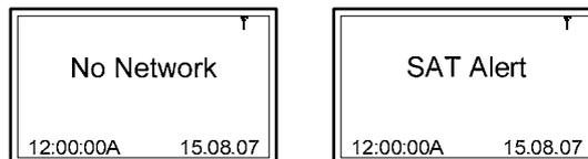
2. If turning on the Main Unit without using the SIM card, the following message will be displayed. In this case, user should turn off the power, insert the SIM card into the Main Unit and then turn on the power again.
