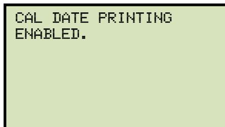
The calibration date printing option will be enabled and you will be returned to the "START-UP" menu. Figure 3 shows a sample test report with the calibration expiration date printed at the bottom.
