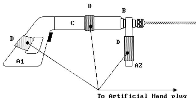
Fig. 5-2 Typical hand held equipment test set-up
