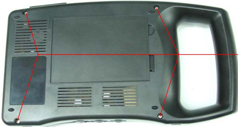
Screw off these 4 screws with Phillips screw driver.
