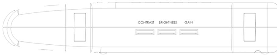
Figure 1-8 WED-2000AV underside turn-button sketch map
