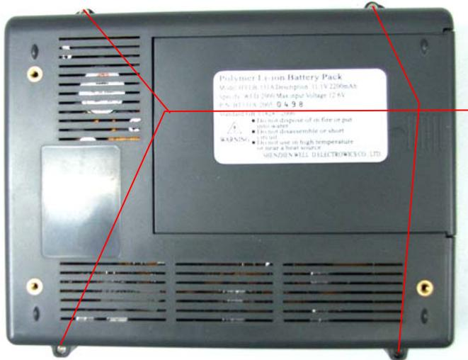
Screw off these 4 screws with Phillips screwdriver.
