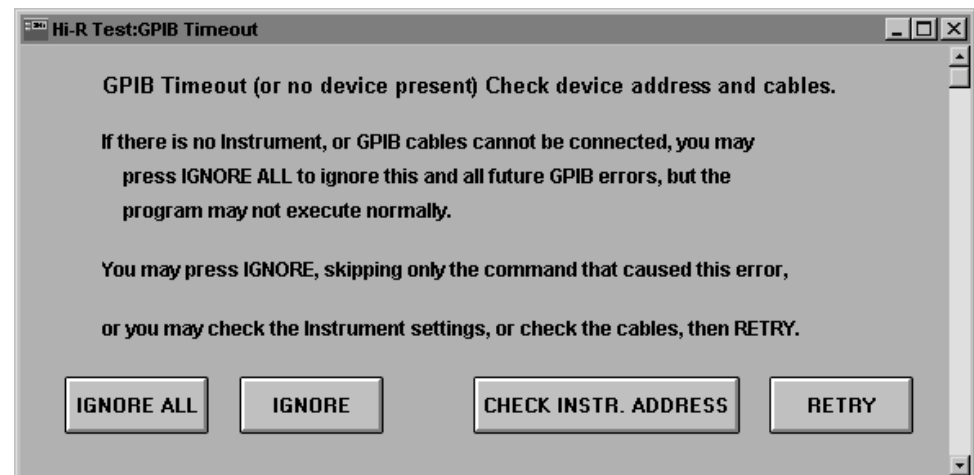
Figure 1-8 GPIB timeout panel
