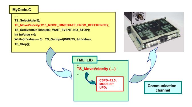
Figure 1.1. Using TML\_LIB to control a Technosoft intelligent drive from the PC computer
