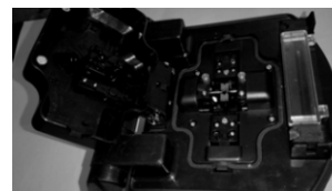
Figure 5-1.1: Fiber holder FH-35-125-R-A for covered wire
