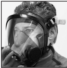
FACE SEAL ROLLED OVER
