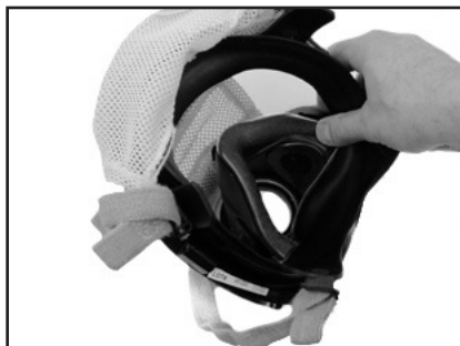
FIGURE 1 Checking Voicemitter Ducts
