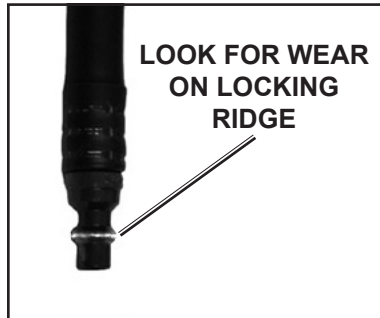
FIGURE 5 Inspecting Male Quick Disconnects
