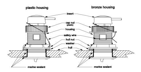
Figure 3 - Bedding and Installation
