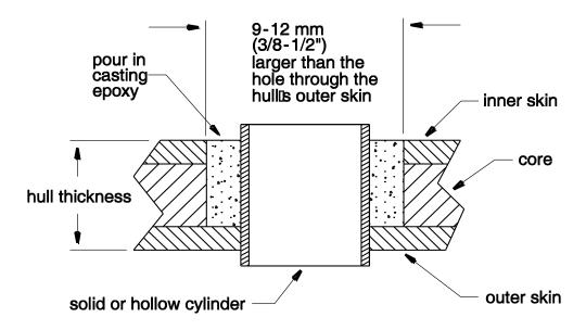
Figure 4 – Preparing a Cored Fiberglass Hull
