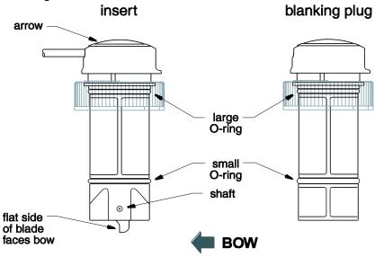
Figure 6 – Replacing the Paddlewheel and O-rings
