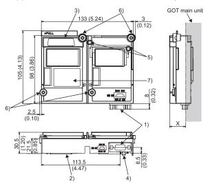
Dimensions of X when the RGB output unit is mounted to the GOT.
