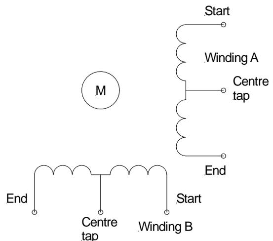
Figure 6. 6-wire motor
