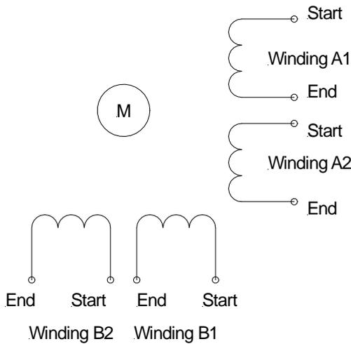
**Figure 7. 8-wire motor**
