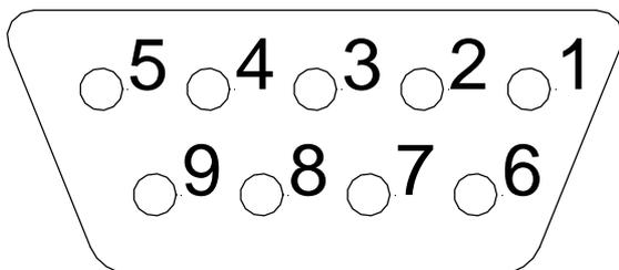
Figure 12. “D”-type socket pinout
