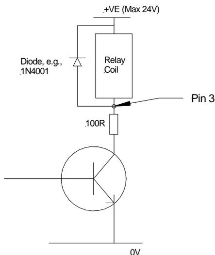
**Figure 13. Using “Active/Inactive” to drive a relay**
