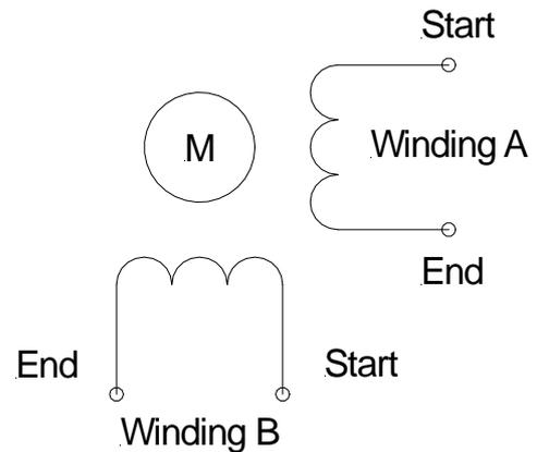
Figure 5. 4-wire motor
